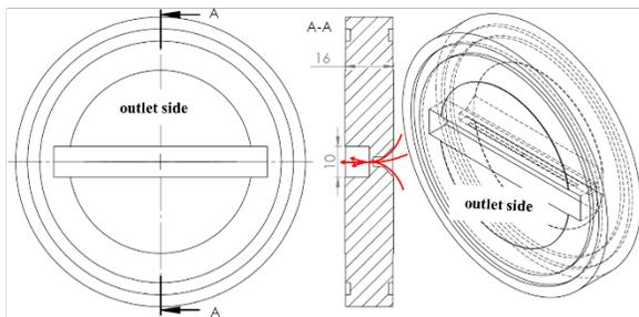
Figure 4. Technical drawing of specimen with pin hole, defined slit and fatigue crack
