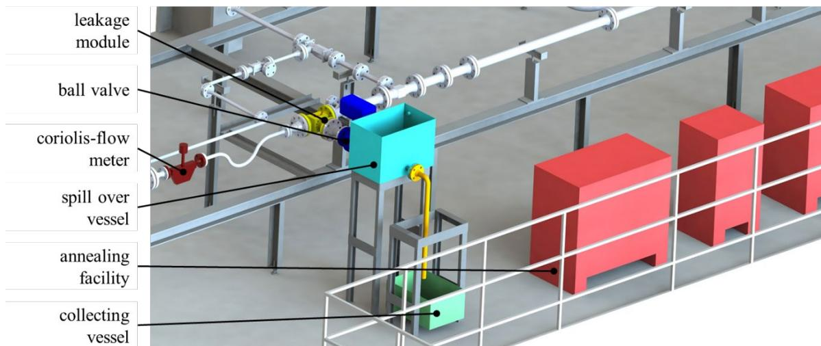
Figure 3. FSI test rig configuration for investigation of discharge into water
