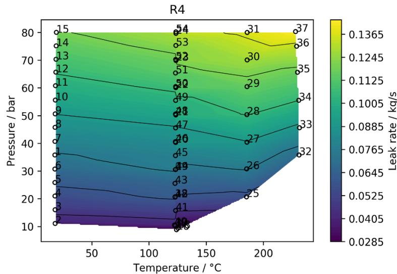
Figure 8. Measured leak rates at specimen R4
