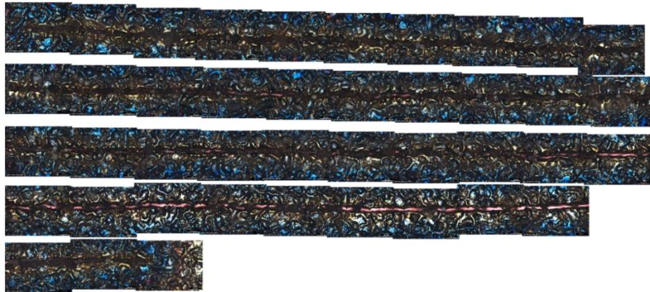
Figure 5. Stitched images of the fatigue crack of R4 from the inlet side after leak rate measurement with a full crack length of around 42 mm
