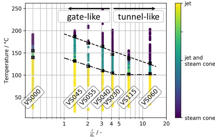
Figure 12. Flow pattern dependent on relative flow length ( $l/d_h$ )
