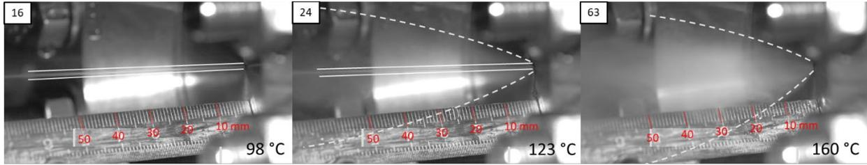
Figure 9. Flow pattern at around 50 bar for specimen VS030 at 98 °C, 123 °C and 160 °C
