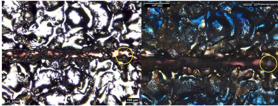
Figure 7. Image of the inlet at specimen R4 before (left) and after (right) leak rate measurement with particle from PIV measurements
