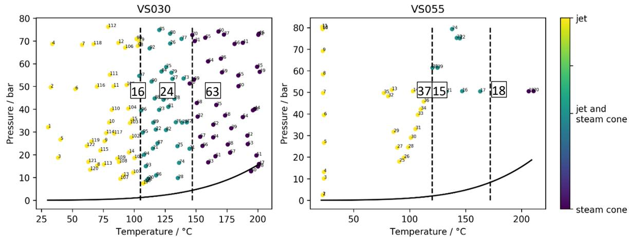
Figure 11. Categorization of discharge flow pattern for specimen VS030 and VS055, the numbers in squares refer to the numbers in Figure 12 and Figure 13.
