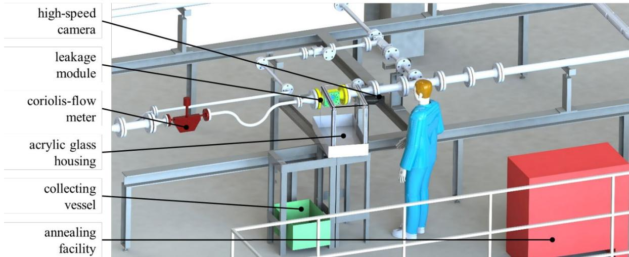
Figure 2. FSI test rig configuration for optical investigation (free discharge, high-speed camera)
