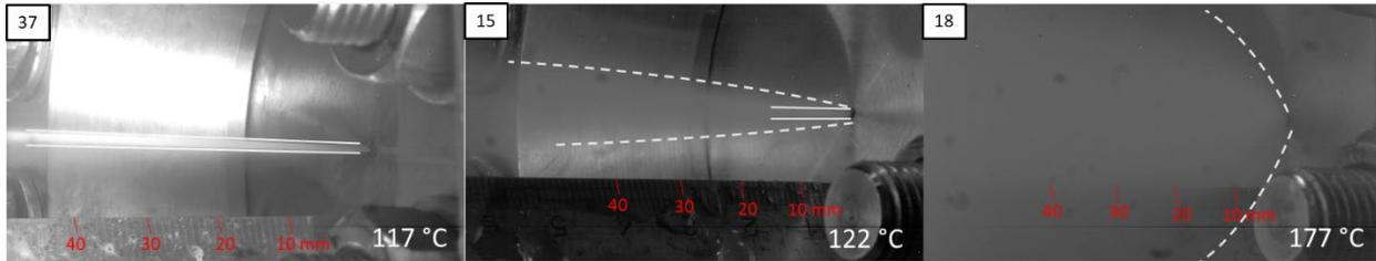
Figure 10. Flow pattern at around 50 bar for specimen VS055 at 117 °C, 122 °C and 177 °C
