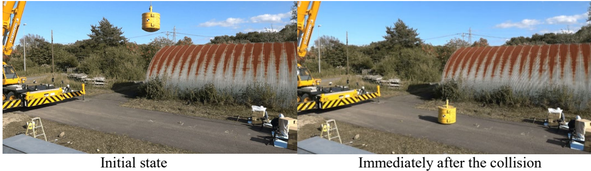
Figure 4. Vertical drop test of specimen (asphalt pavement)
