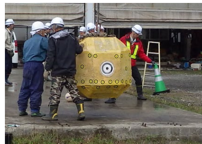
EOTA type test piece (1.6t in this picture)
