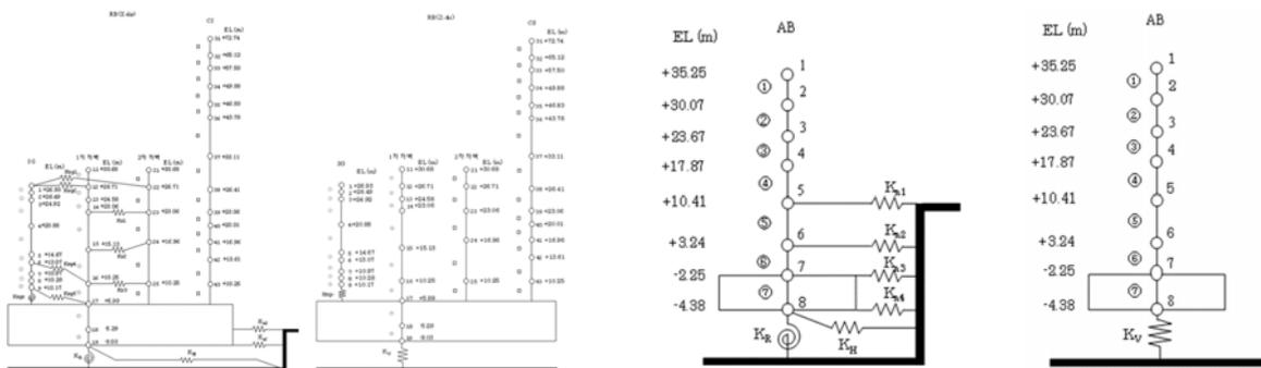
Figure 7. Lumped mass stick models of horizontal and vertical direction for RCB and AB
