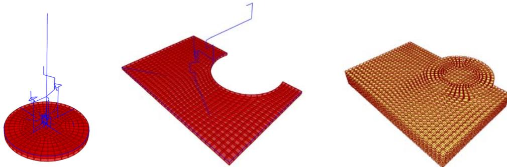
Figure 6. Lumped mass stick models of RCB, AB and soil foundation
