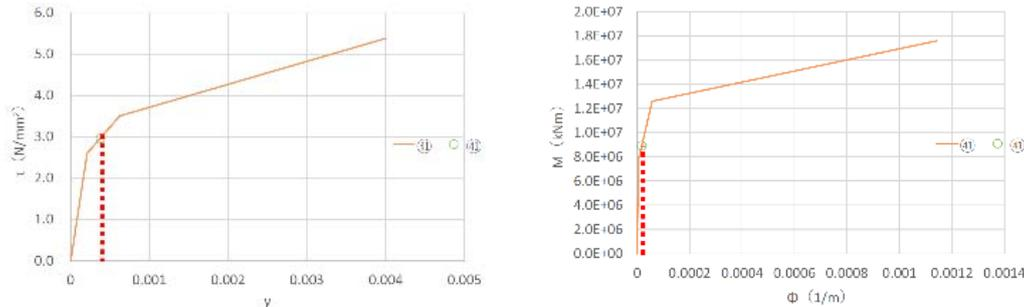
Figure 9. Shear strain and moment curvature levels at RCB wall
