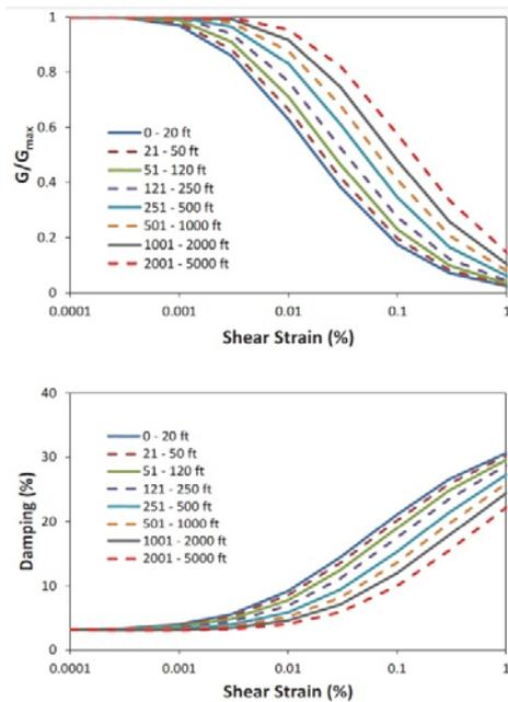
Figure 3. Nonlinear characteristics of rock
