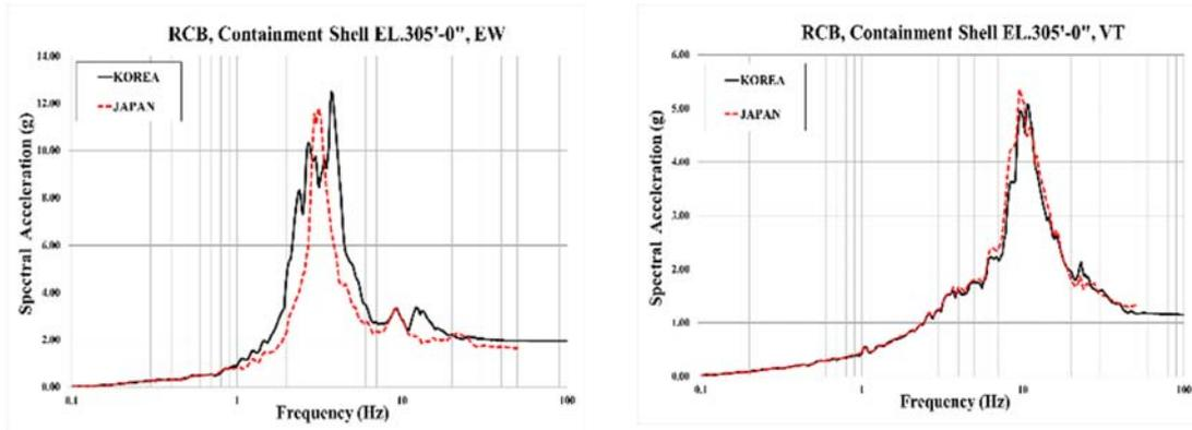
Figure 8. Floor responses spectra in horizontal and vertical directions at RCB dome apex
