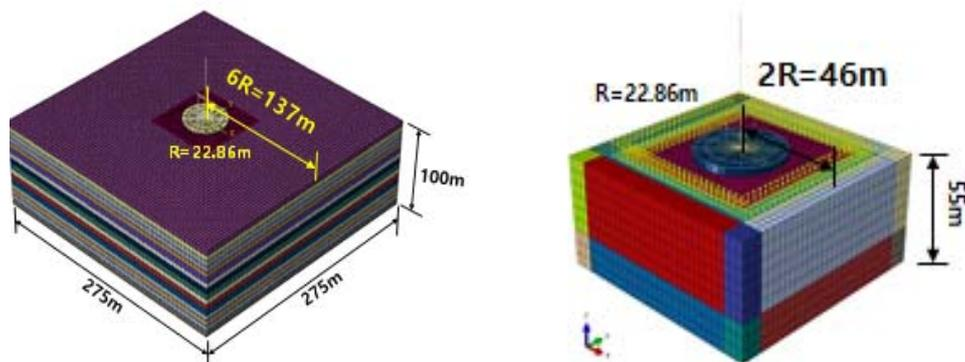
Figure 13. DM model and DRM-PML model for the nonlinear analysis of the RCB
