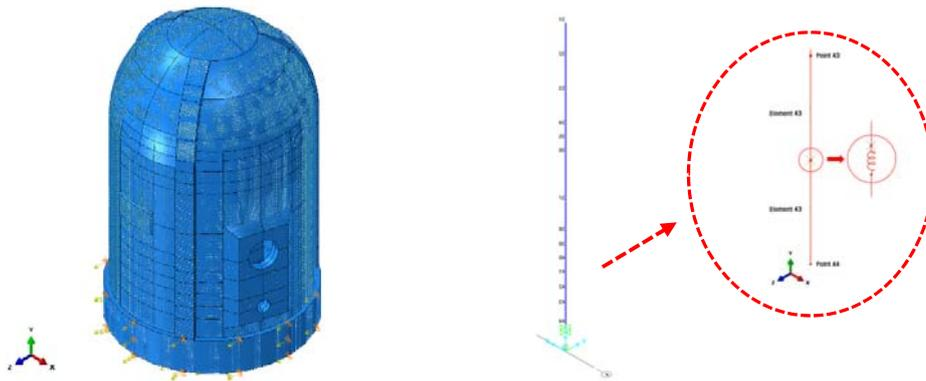
Figure 11. FE model and beam stick model for the RCB
