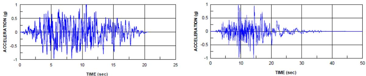
Figure 1. Horizontal acceleration time histories according to design requirements of SRP 3.7.1 and JEAG 4601
