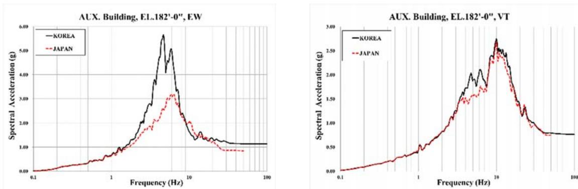
Figure 10. Floor responses spectra in horizontal and vertical directions at AB roof
