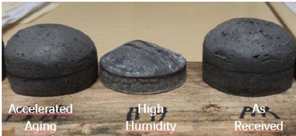
Figure 2 : intumescent material tested according to the UL1459 standard. The “as received” and aged specimens were expanded in an oven at 300°C for 30 min
