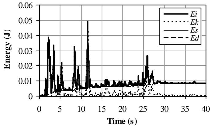
Figure 3. Energy response of seismometer with  $\beta = 2/\pi$ .
