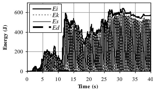
Figure 2. Energy response of elastic SDOF system with  $\beta = 0$ .
