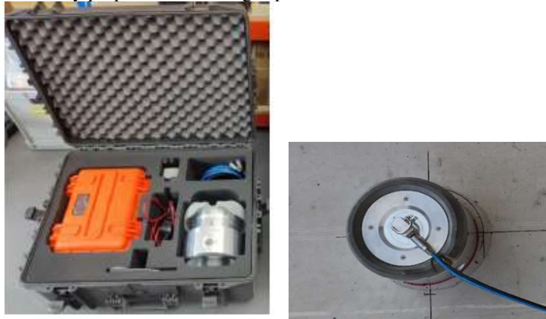
Figure 5. Left: Installation tooling in its box – Right: installation bell during bonding.
