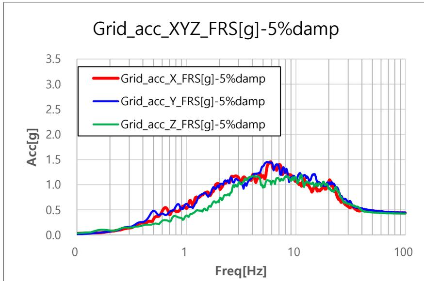
a) FRS2 at Grid Plate of Full FE Model
