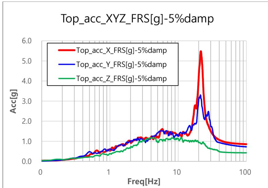
a) FRS2 at Reactor Cover Plate of Full FE Model
