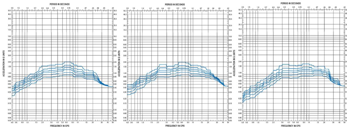
Figure 2 Enveloped 18 case FRS1 (EW-x, NS-y, VT-z, and 2, 3, 4, 5, 7, 10% damping)
