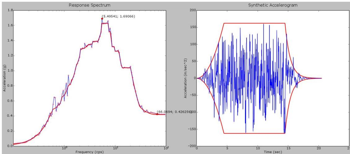
Figure 3 Comparison of calculated Spectra (3% damping) with given FRS1 at Reactor Assembly Bottom and its Artificial Time History in EW x-direction
