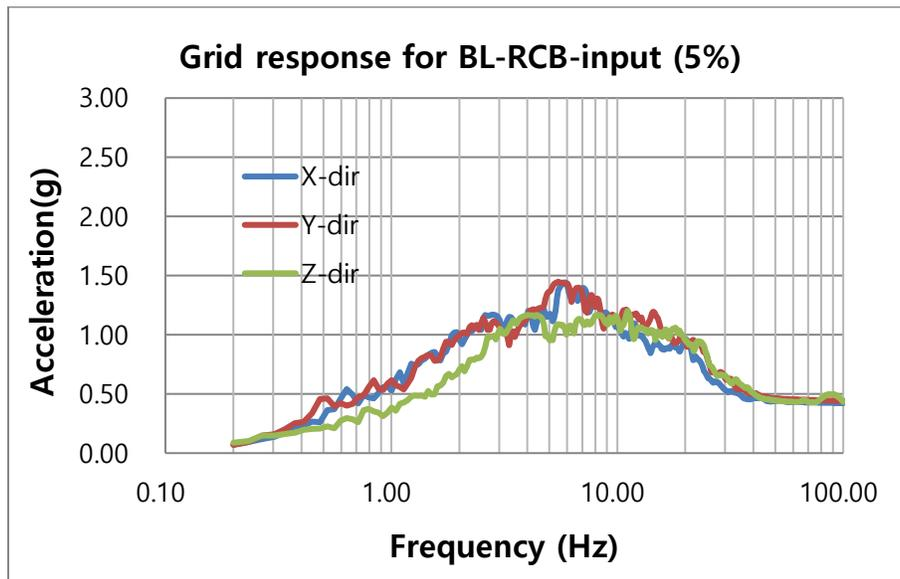
b) FRS3 at Grid Plate of Simplified FE Model
