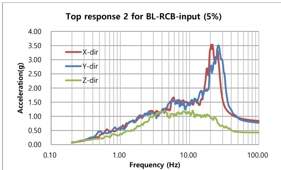
b) FRS3 at Reactor Cover Plate of Simplified FE Model
