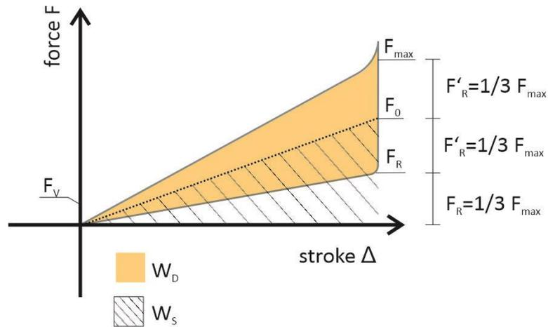
Figure 5. Work done,  $W_S$  work of stiffness,  $W_D$  work of damping (Helm, L., Sadegh-Azar, H., Jahnelt, L., Jandrey, H. 2022)
