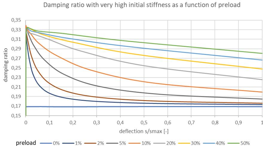
Figure 6. Damping ratio as a function of preload (Helm, L., Sadegh-Azar, H., Jahnel, L., Jandrey, H. 2022)
