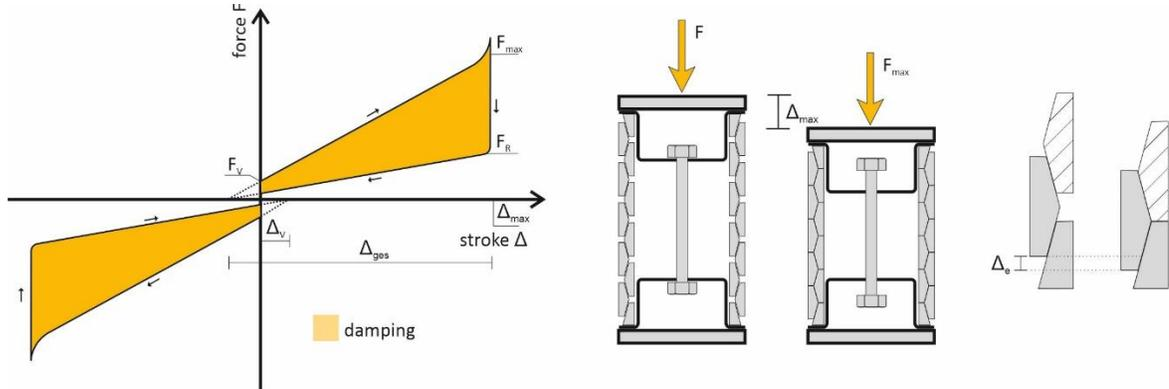
Figure 1. Design and typical load-deformation curve of a ring spring (Helm, L., Sadegh-Azar, H., Jahnel, L., Jandrey, H. 2022)
