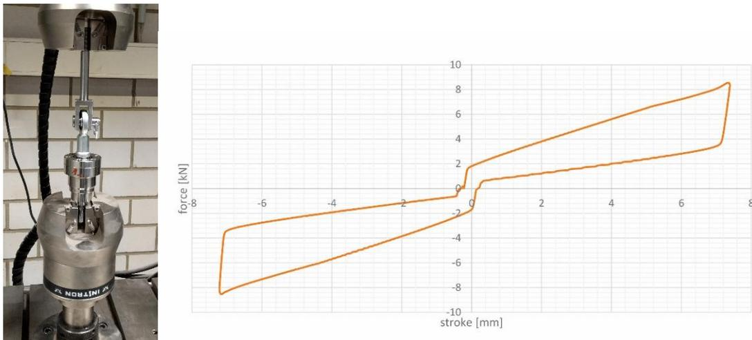
Figure 3. Load-deformation measurement of a double-acting ring spring
