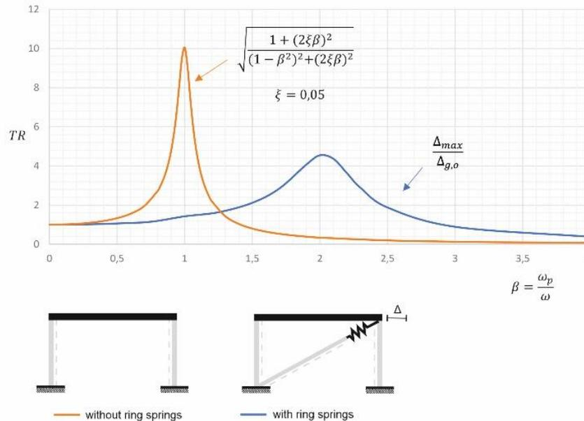
Figure 8. Magnification function of a system with and without ring springs (Helm, L., Sadegh-Azar, H., Jahnel, L., Jandrey, H. 2022)
