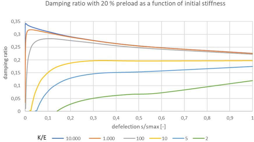
Figure 7: Damping ratio as a function of initial stiffness (Helm, L., Sadegh-Azar, H., Jahnelt, L., Jandrey, H. 2022)
