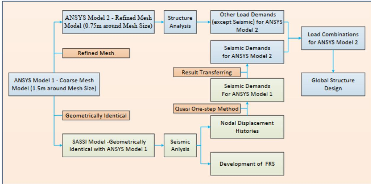
Figure 2. Data transfer between various models
