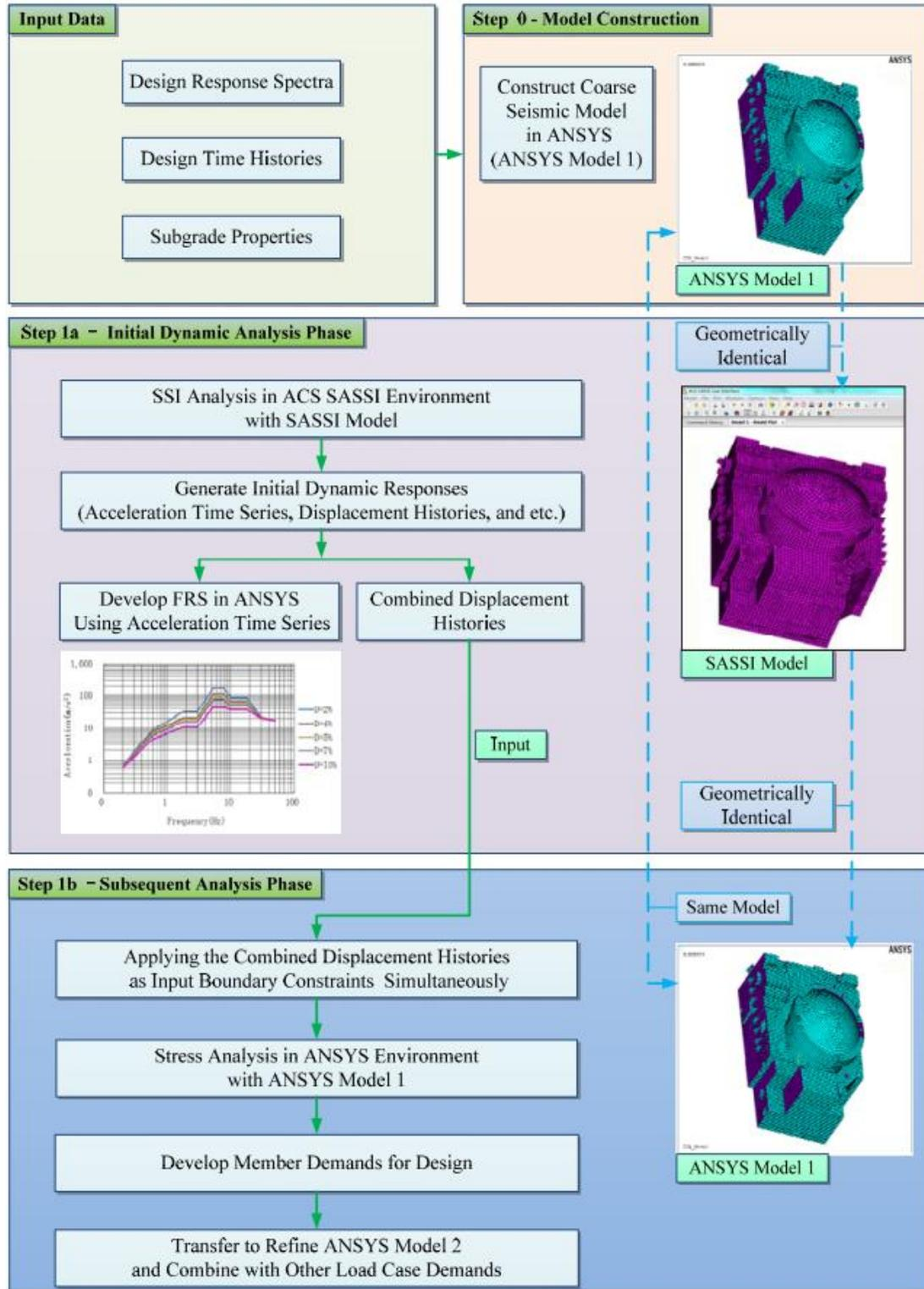
Figure 1. Overall Seismic Analysis Approach
