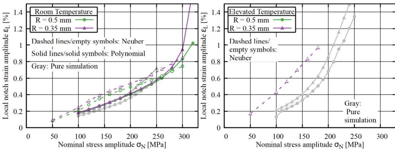
Figure 8. Local notch root strain as a function of the nominal stress amplitude
