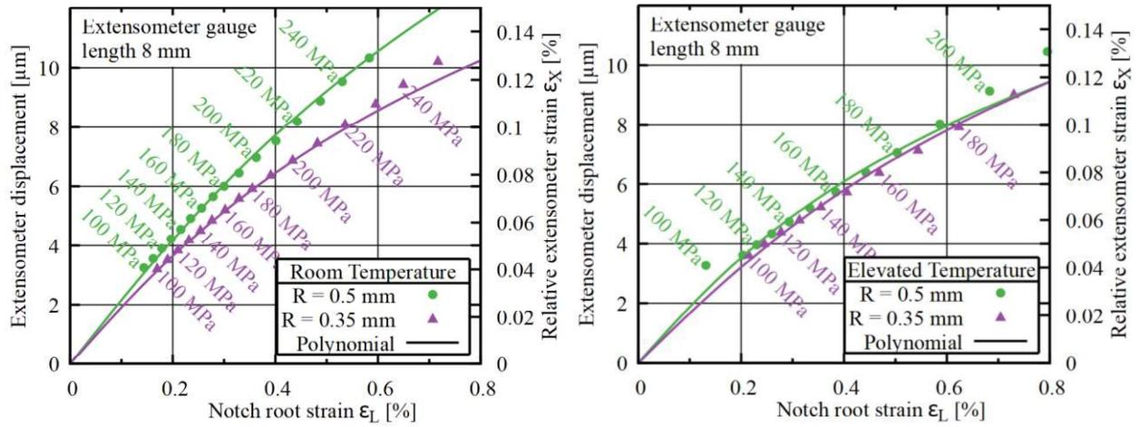
Figure 6. Relation between FE-calculated notch root strain and FE-calculated extensometer strain for the 0.5 mm notch and the 0.35 mm notch for room temperature (left) and elevated temperature (right).
