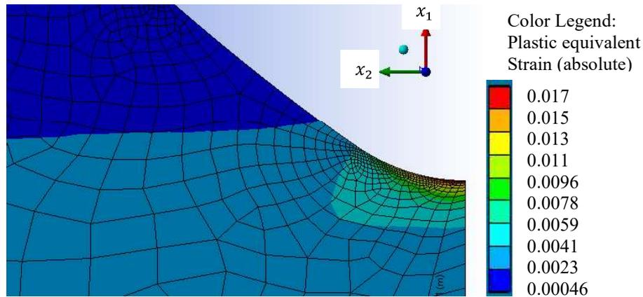
Figure 5. Finite Elements Analysis of the notched specimen:
