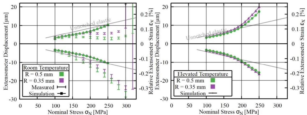
Figure 7. Measured extensometer strain for different nominal stresses (bars indicating the range on each stress level) and comparison with the simulation (line-connected points).
