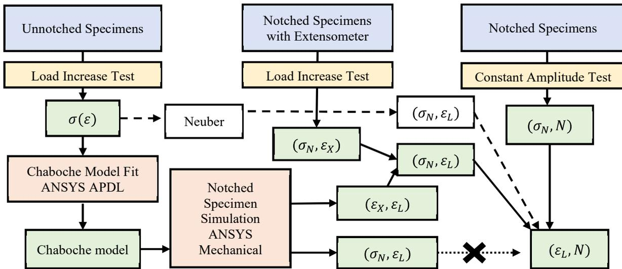
Figure 10. Flow chart of the assessment of notched fatigue specimens.
