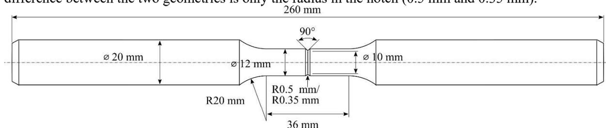
Figure 3. Specimen geometry with two different notch radii
