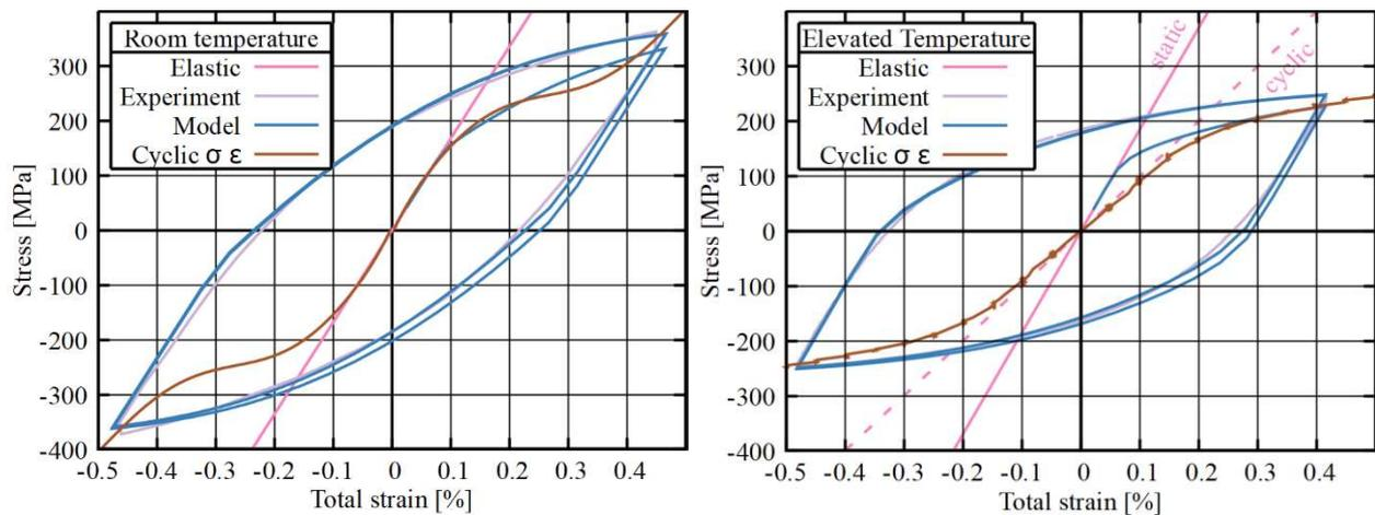
Figure 2. Stress-strain relation and fitting result of the plasticity model at the two temperature levels
