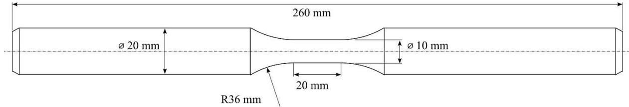
Figure 1. Geometry of unnotched specimen.
