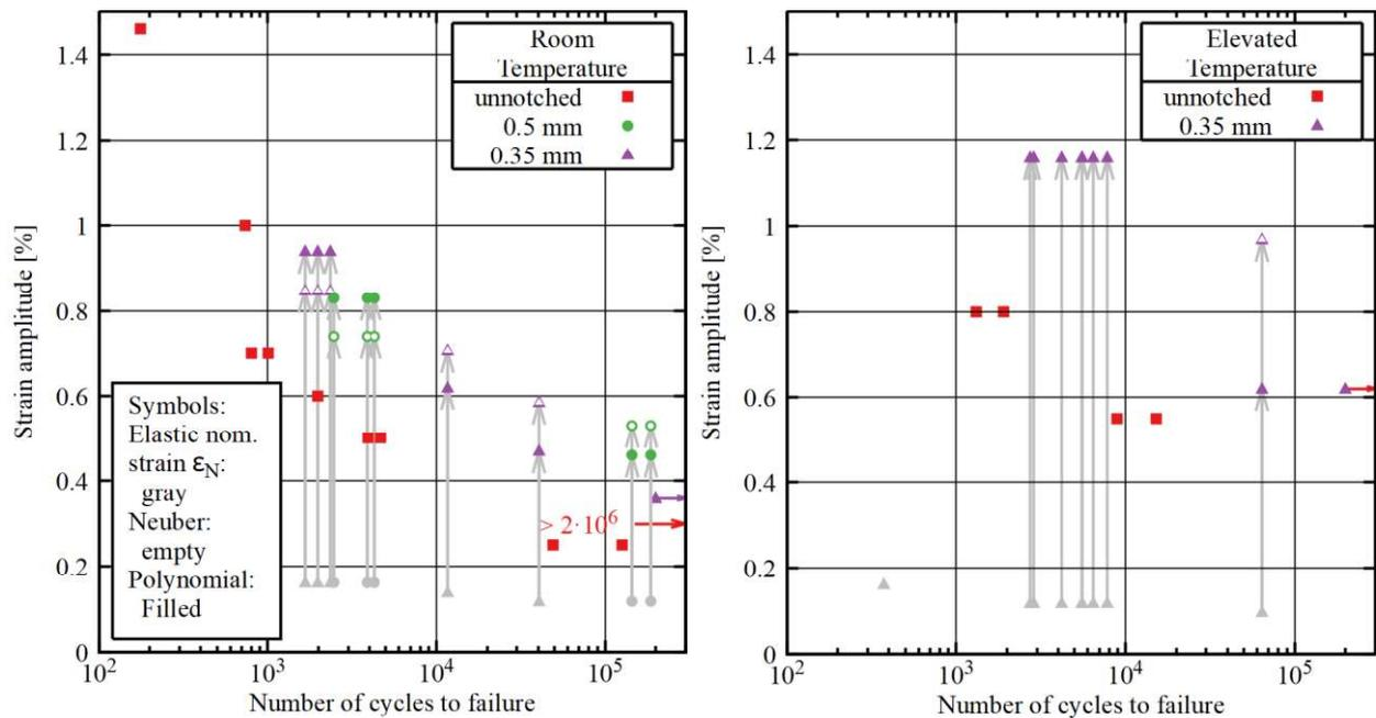
Figure 9. Fatigue diagrams at room temperature (left) and elevated temperature (right).
