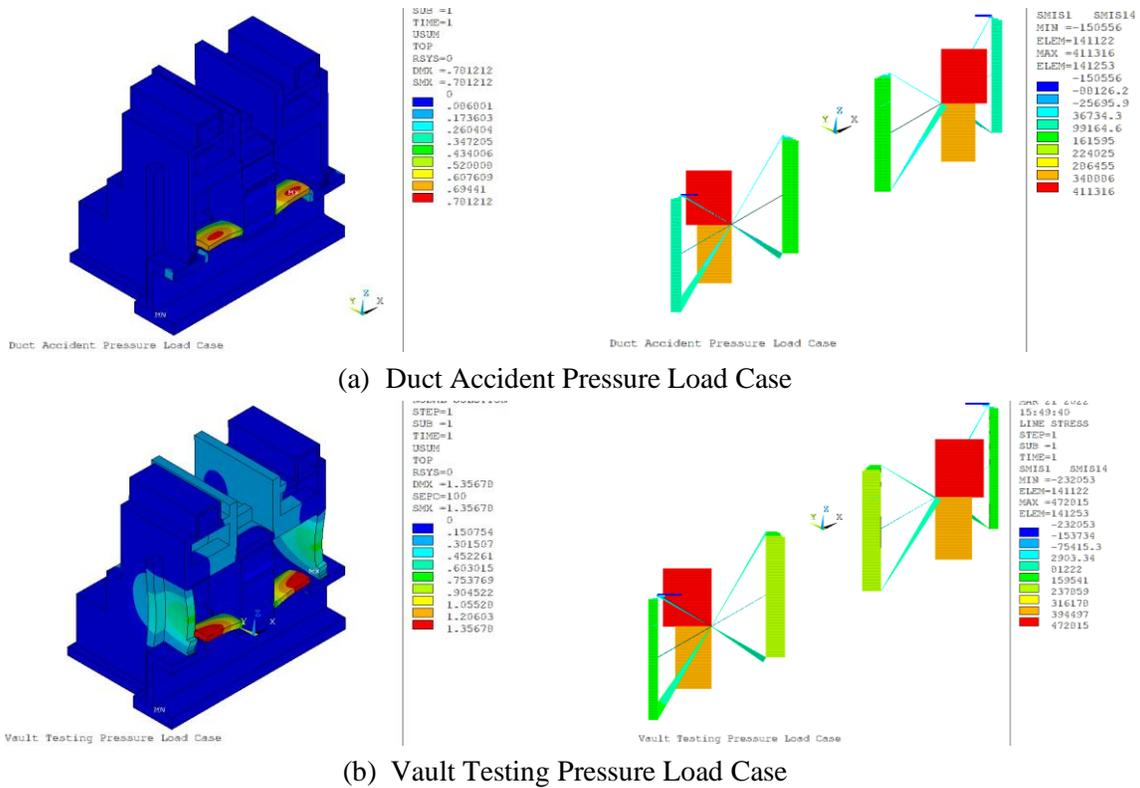
Figure 8. Vault Deformation & Column Tension Response using Coupled Analysis Model
