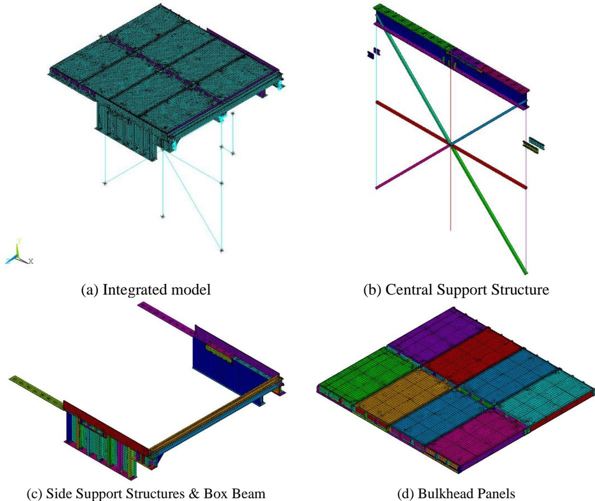
Figure 4. Numerical Model of The Containment Isolation System
