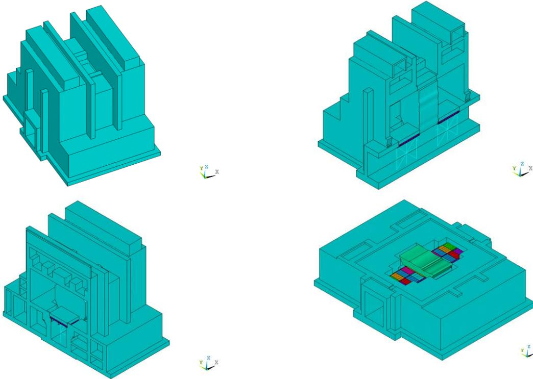
Figure 7. Coupled Analysis Model of Isolation System/Vault
