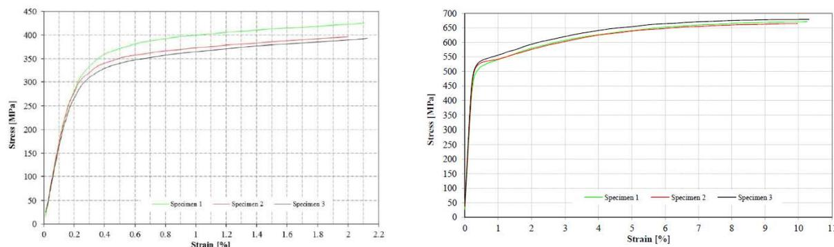
Figure 4. Tensile test results on missile specimen (on the left) and rebar specimen (on the right)
