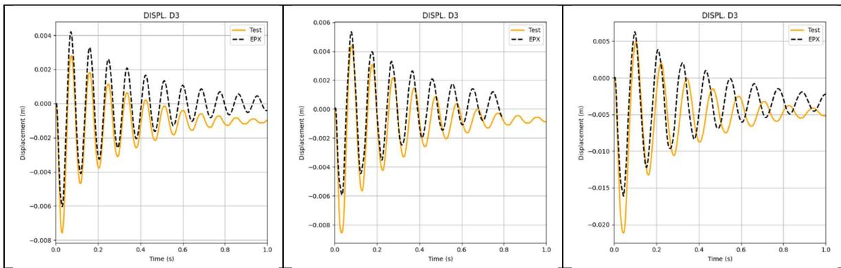
Figure 6. Displacements at sensor D3 for impact 1 (on the left) to impact 3 (on the right)
