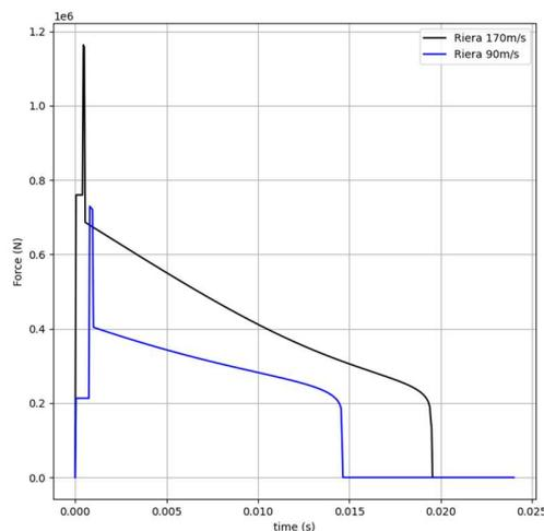
Figure 3 : Impact loading for tests Va / Vb (90 m/s) and Vc (170 m/s)
