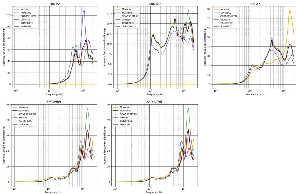
Figure 12. Sensitivity study – FRS at A2, A3H, A7, A9B and A9W for the third impact
