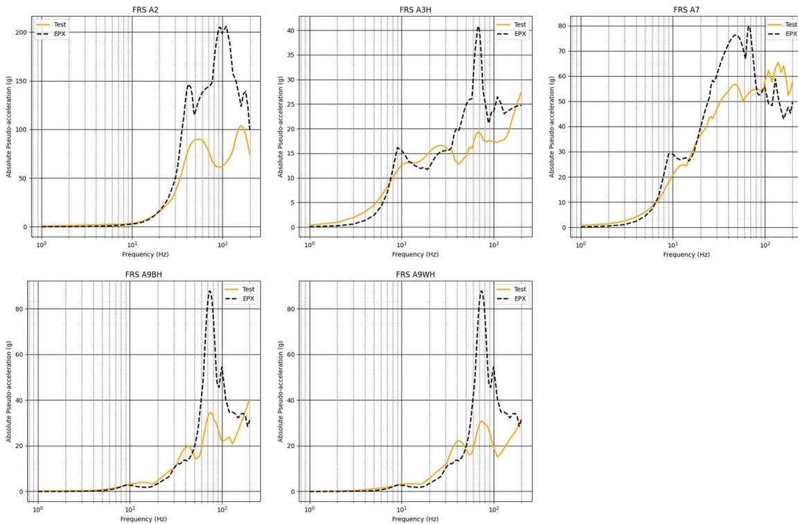
Figure 11. FRS at sensors A2, A3H, A7, A9BH and A9WH for the third impact
