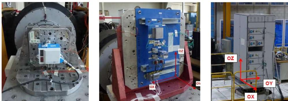
Figure 14. EDF HF testing program – Some of the tested electrical equipments (temperature sensor on the left; relay command board at the centre; LT switchboard on the right)
