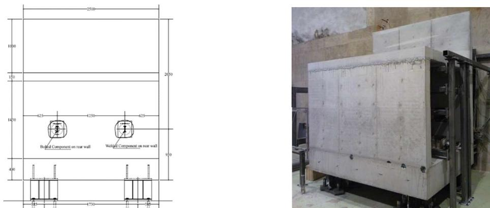
Figure 2. IRIS 3 mock-up (front view) from a drawing and a photo in the test hall
