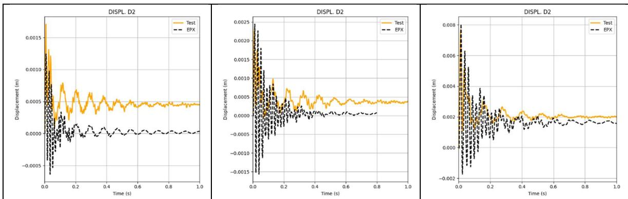
Figure 7. Displacements at sensor D2 for impact 1 (on the left) to impact 3 (on the right)
