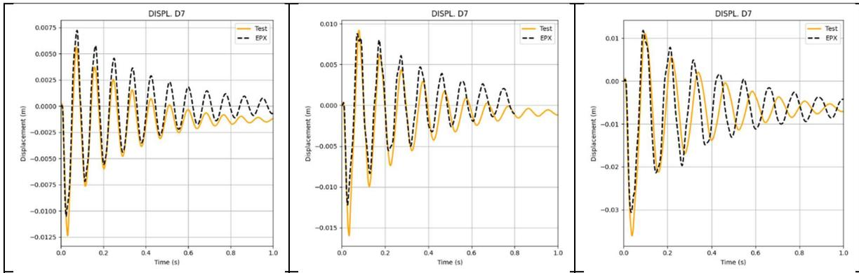
Figure 8. Displacements at sensor D7 for impact 1 (on the left) to impact 3 (on the right)
