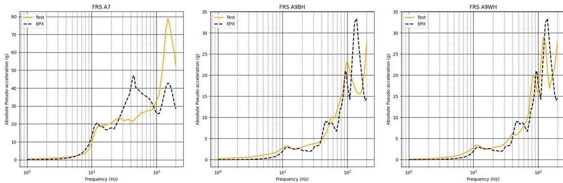
Figure 9. FRS at sensors A7, A9BH and A9WH for the first impact
