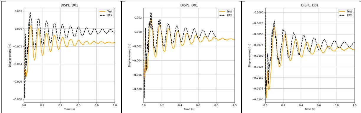
Figure 5. Displacements at sensor D01 for impact 1 (on the left) to impact 3 (on the right)
