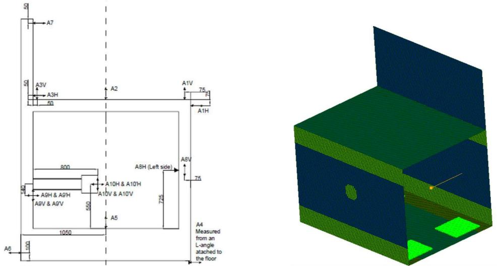
Figure 1. Acceleration sensors A1 to A10 in the mock-up symmetry plane (side view) and view of the FE mesh for numerical calculations. The circle in the figure on the right represents the impact surface
