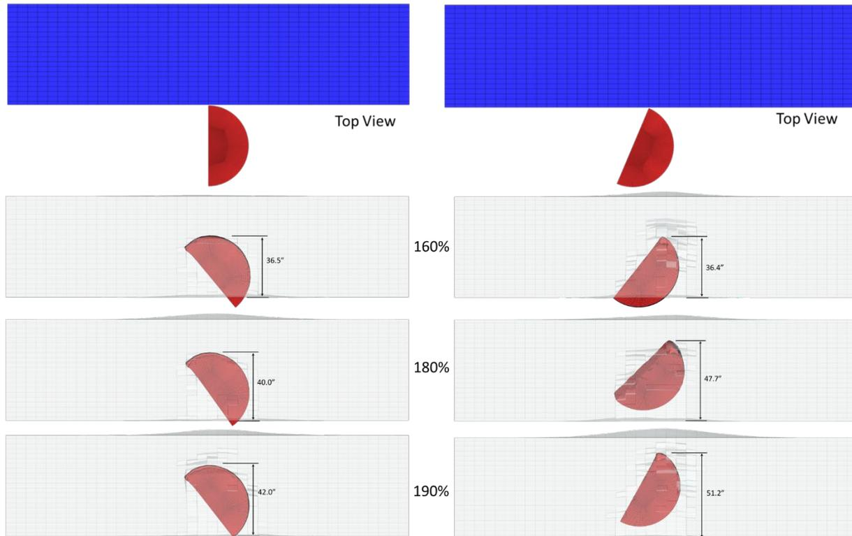
Figure 10. Penetration Depth of Rotor, Perpendicular Alignment (Left) and CG Alignment (Right)
