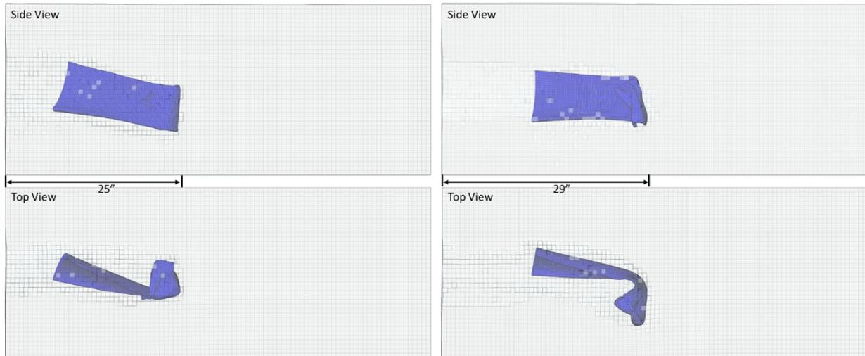
Figure 7. Penetration Depths at 160% Overspeed (Left) and 180% Overspeed (Right)
