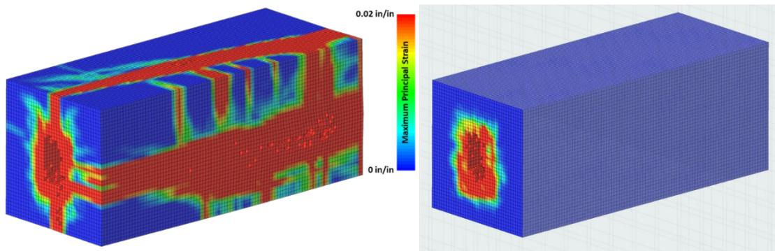
Figure 4. Rigid Blade Impact, Unconfined (Left) and Confined (Right).
