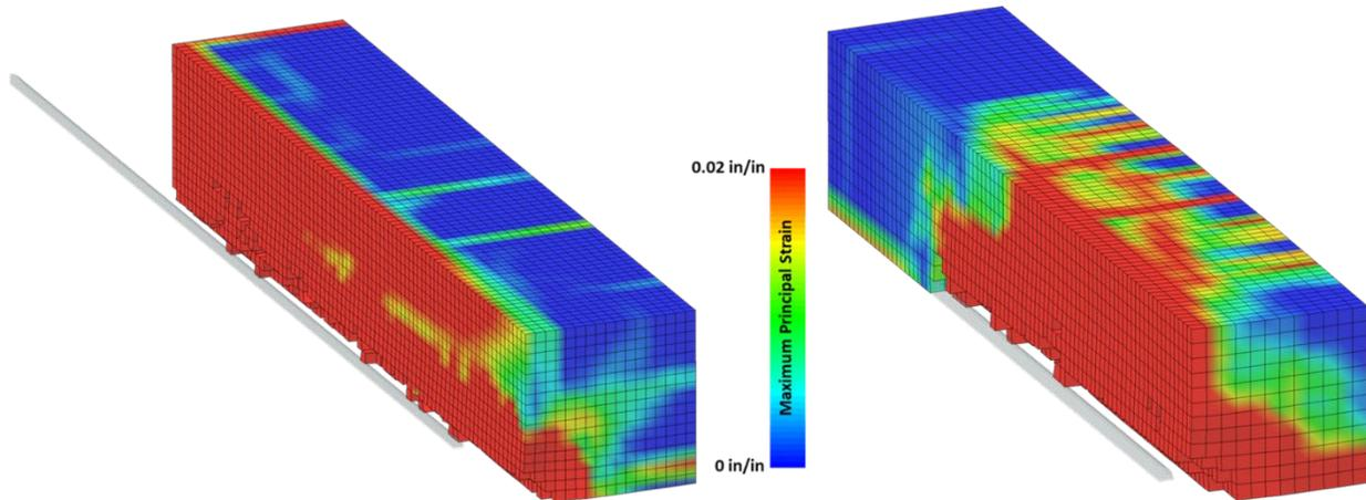
Figure 3. Concrete Strain and Rod Penetration for 1.41” (Left) and 2.0” (Right) Diameter Missiles
