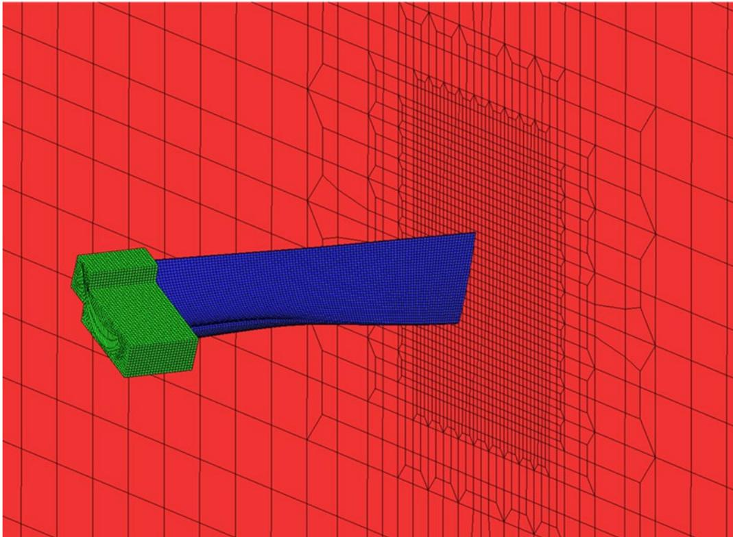
Figure 8. Blade With Root and Concrete Wall Mesh.
