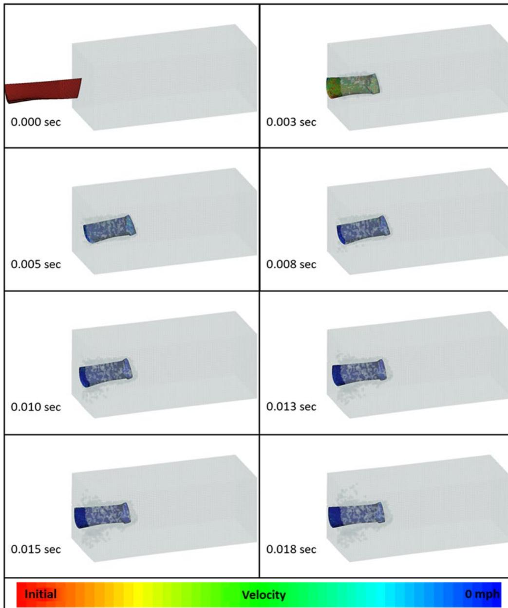
Figure 5. Velocity and Blade Deformation During Impact Simulation
