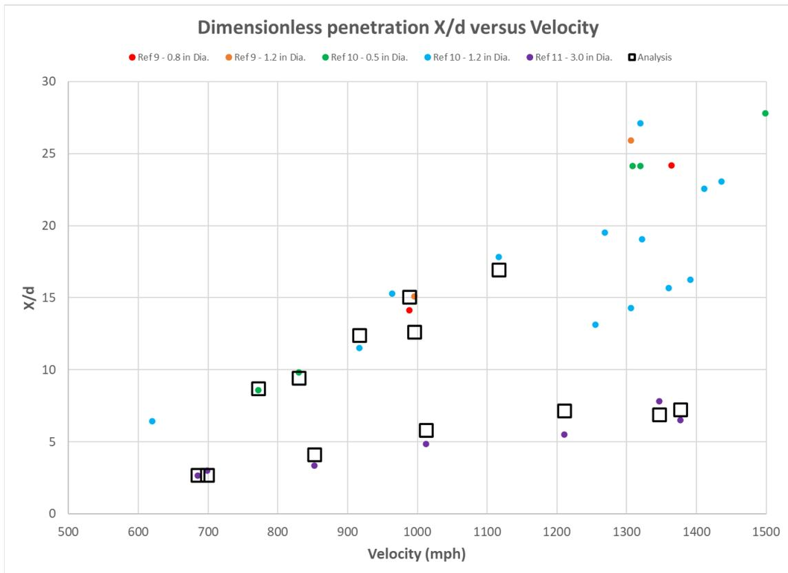
Figure 1. Penetration Depth/Diameter (X/d), Test Data Compared to Analytical Simulation
