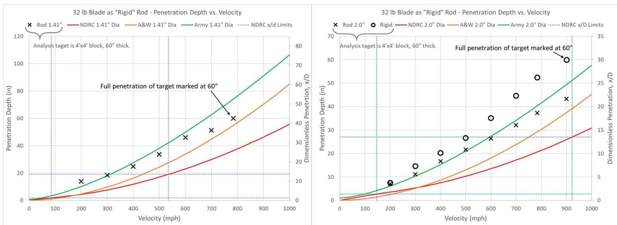
Figure 2. Variable Velocity Penetrations, 1.41-inch Rod (Left) and 2.00-inch Rod (Right)
