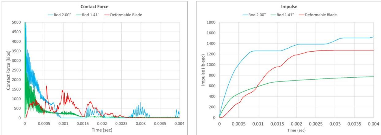
Figure 6. Contact Force (Left) and Impulse (Right) of Impactors Striking a Rigid Wall.
