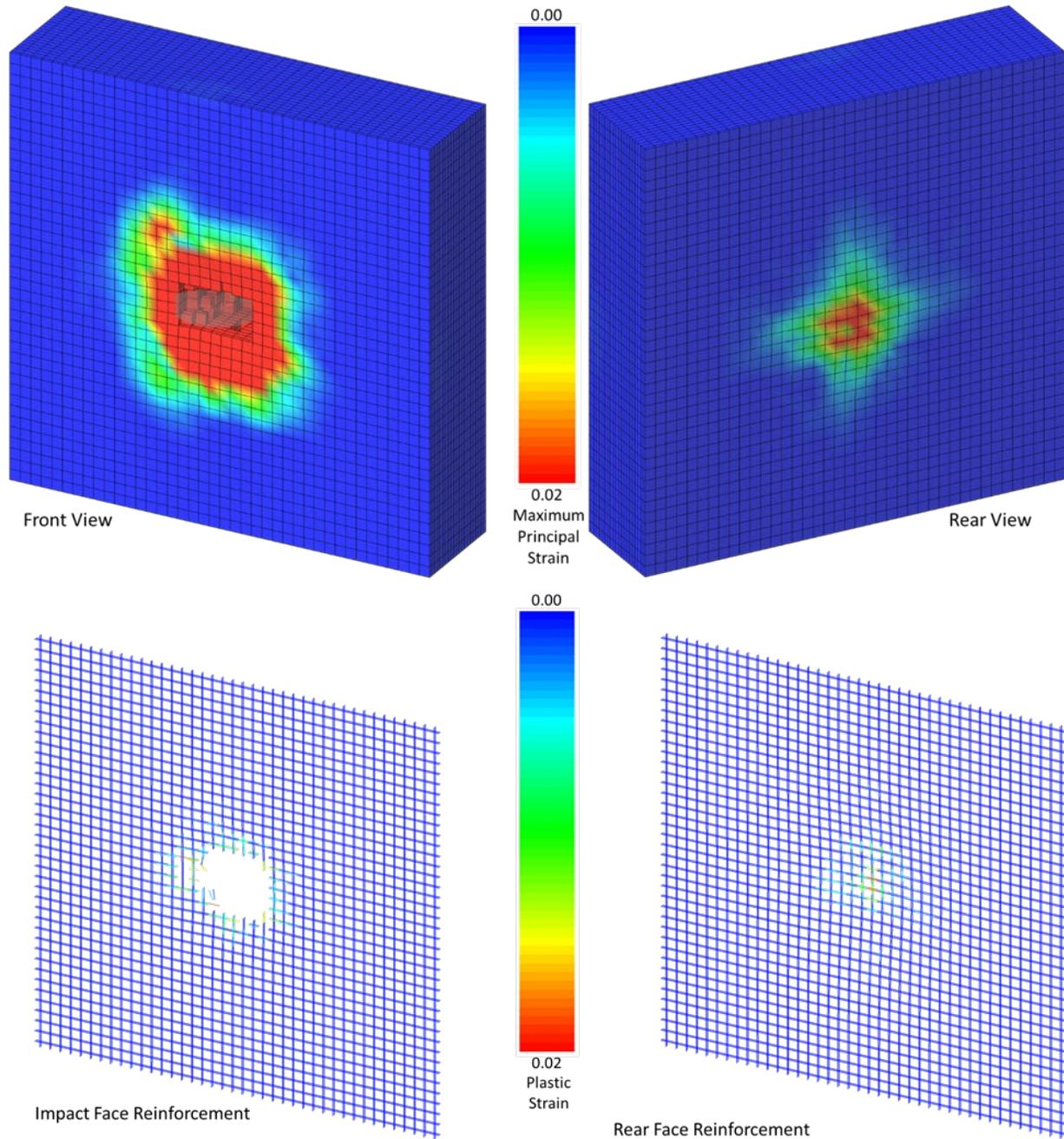
Figure 11. Concrete and Reinforcement Steel Damage With Rotor CG Alignment at 160% Overspeed.
