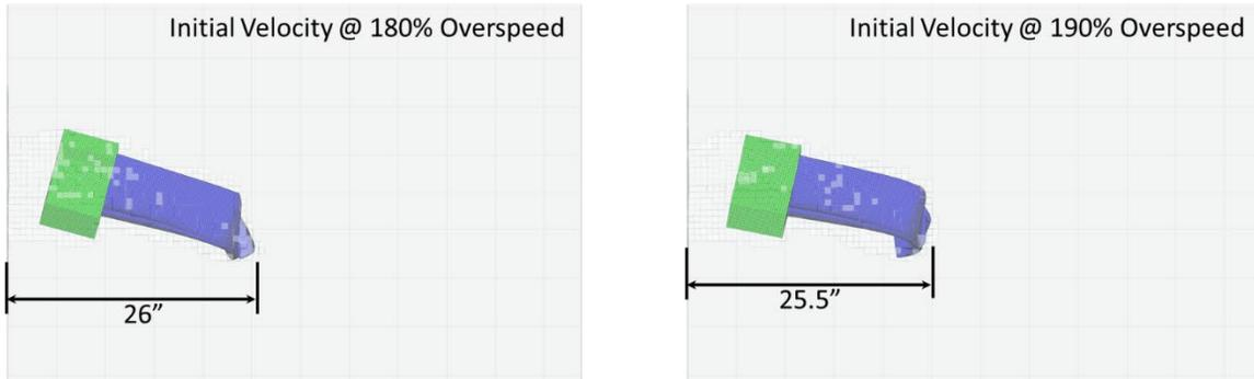
Figure 9. Deformed Blade at Zero Displacement, 180% (Left) and 190% (Right) overspeed cases.
