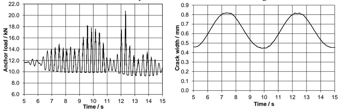
Figure 7. Anchor load (left) and crack width time history (right) during large-scale test with parallel crack configuration
