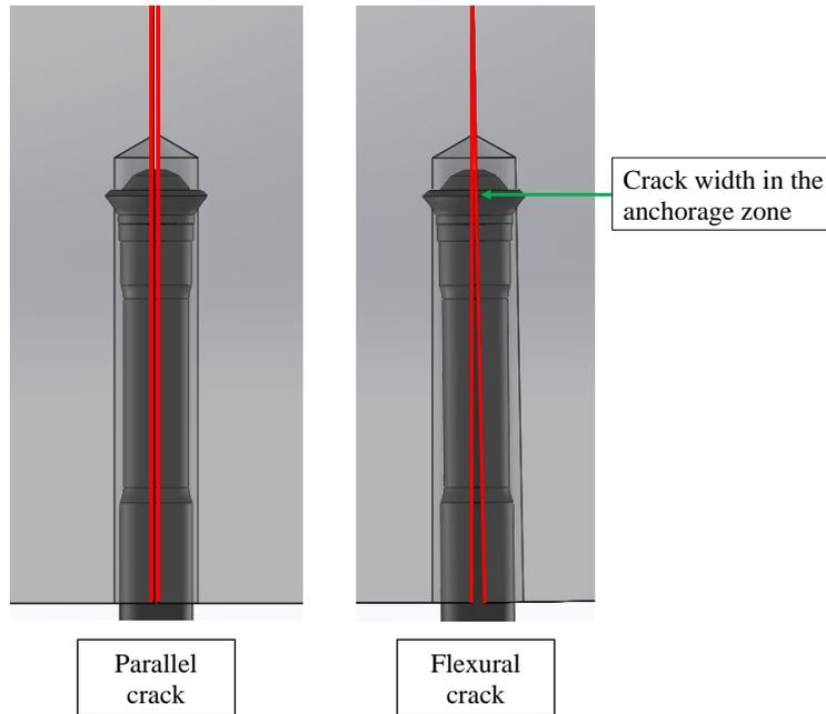
Figure 6. Investigated crack configurations (after [Kerkhof et al. (2017)])
