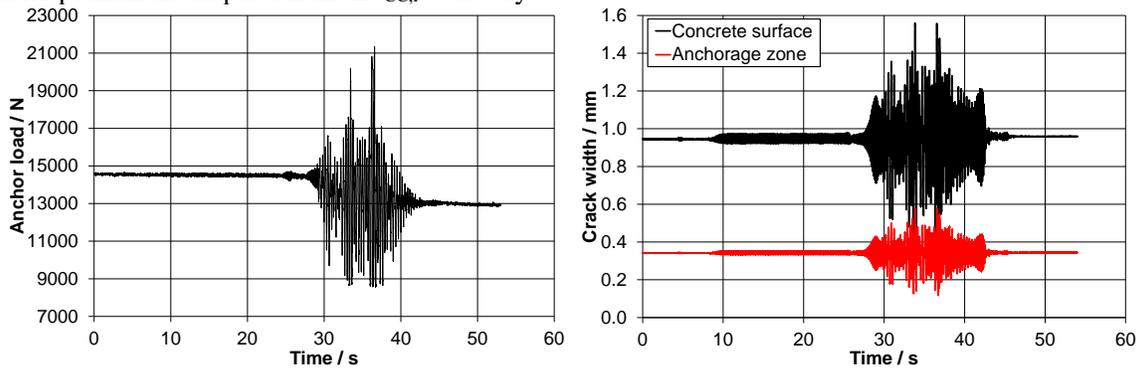
Figure 9. Anchor load (left) and crack width time history (right) during large-scale test with flexural crack configuration
