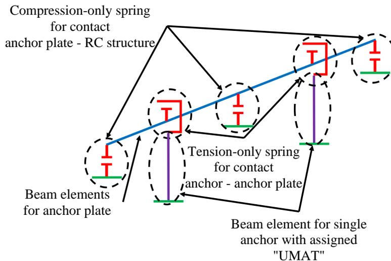
Figure 11. Numerical model of a fastening with two PI anchors (after [Dwenger (2019)])
