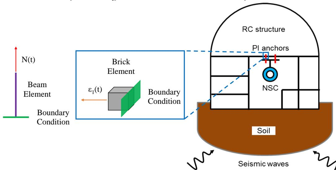
Figure 4. Numerical model of a single anchor
