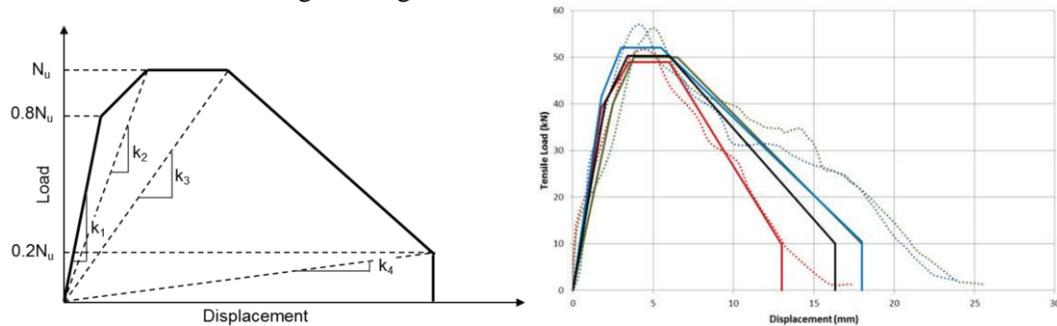
Figure 2. Penta-linear approximation of the load-displacement curve (after [Hofmann, Mahadik and Sharma (2015)])
