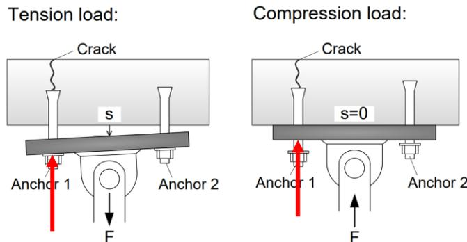
Figure 5. Measurement of anchor plate displacement (red arrow)
