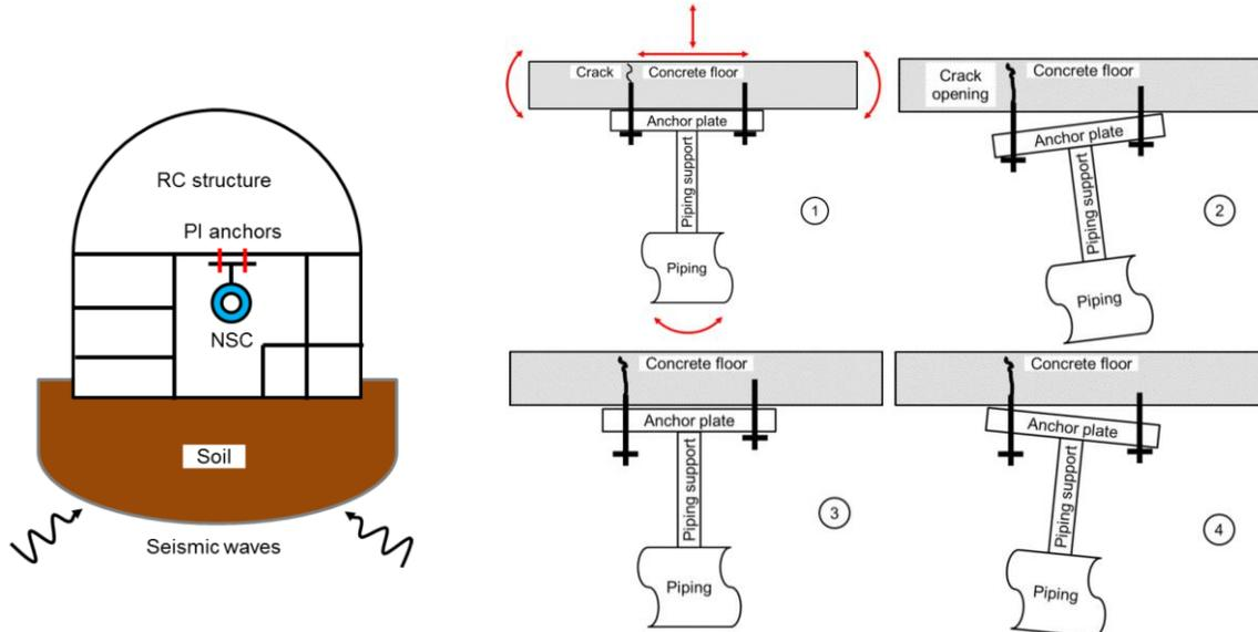
Figure 1. Loading path inside a NPP during an earthquake (left) and behavior of a coupled system during a seismic event (right) (after [Dwenger et al. (2015)], [Dwenger et al. (2017)])
