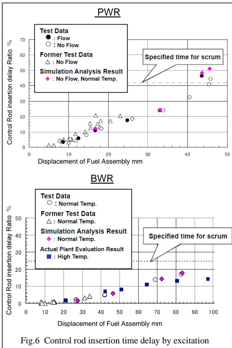
Fig.6 Control rod insertion time delay by excitation
