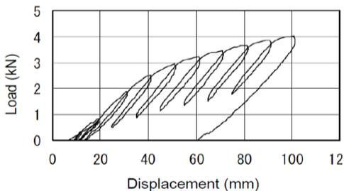
Fig. 5 BWR Control Rod Force-Displacement characteristics
