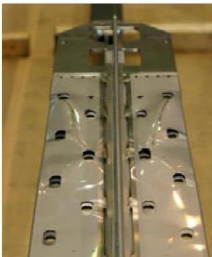
Fig. 4 BWR Control Rod surface Deformation at 3 S<sub>2</sub>
