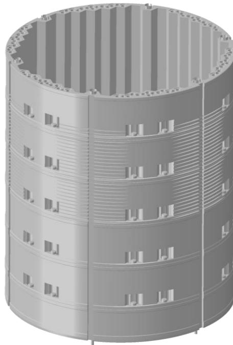
Figure 1. CAD model of the core shroud
