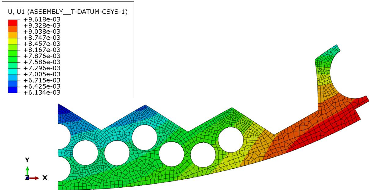
Figure 9. Distribution of radial displacement due to irradiation swelling for 60 years of reactor operation in full power state (in m)
