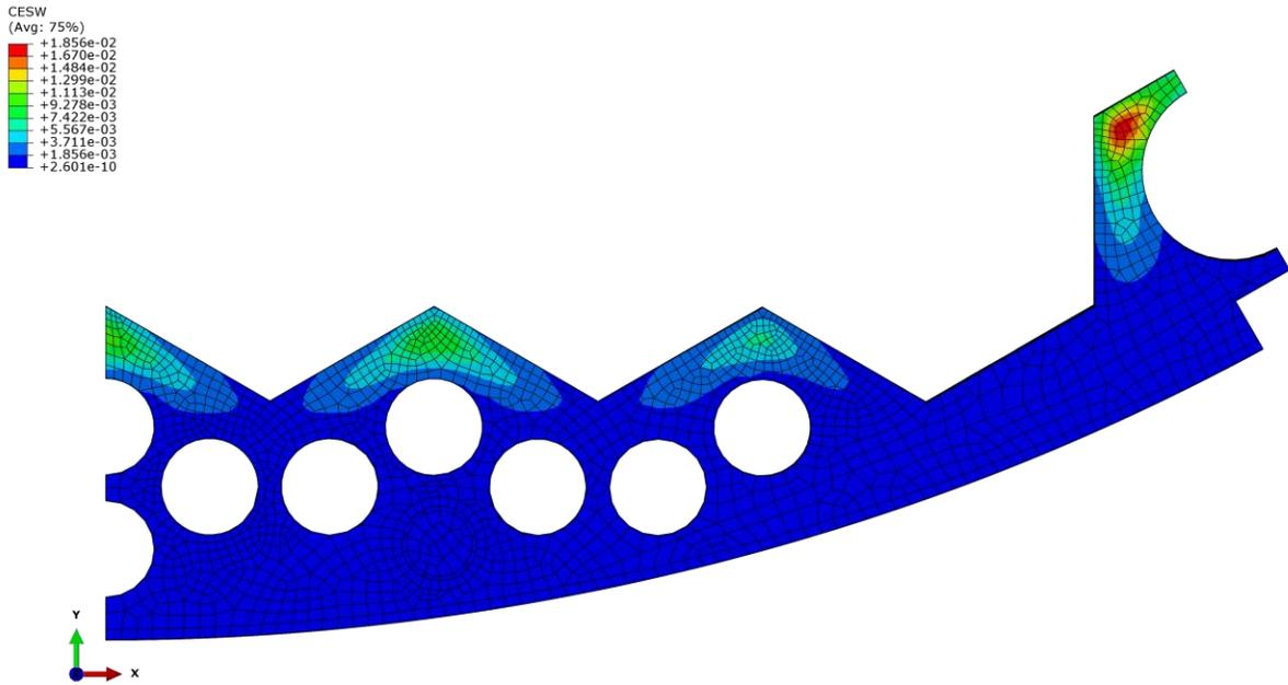
Figure 8. Distribution of volumetric swelling strain (calculated with effect of creep) due to irradiation swelling for 60 years of reactor operation
