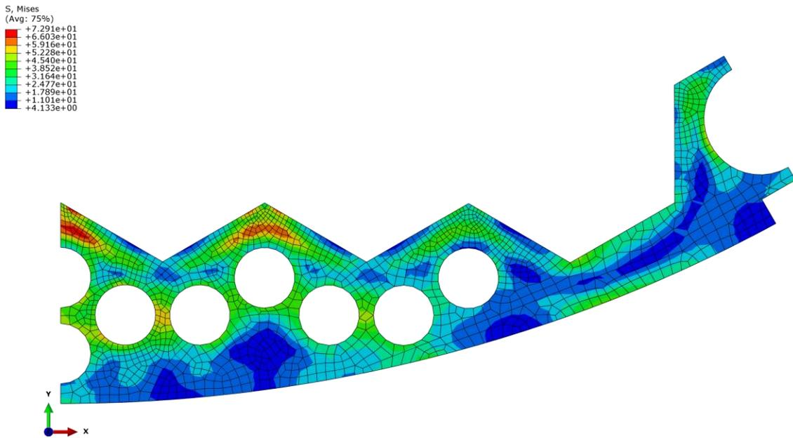
Figure 6. Distribution of von Mises stress for 60 years of reactor operation, for reactor full power state (in MPa)
