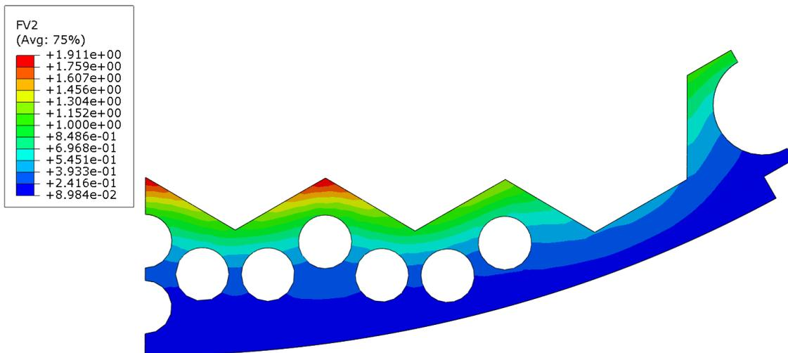
Figure 4. Distribution of neutron dose per selected campaign in cross-section with maximum temperature (in d.p.a.)
