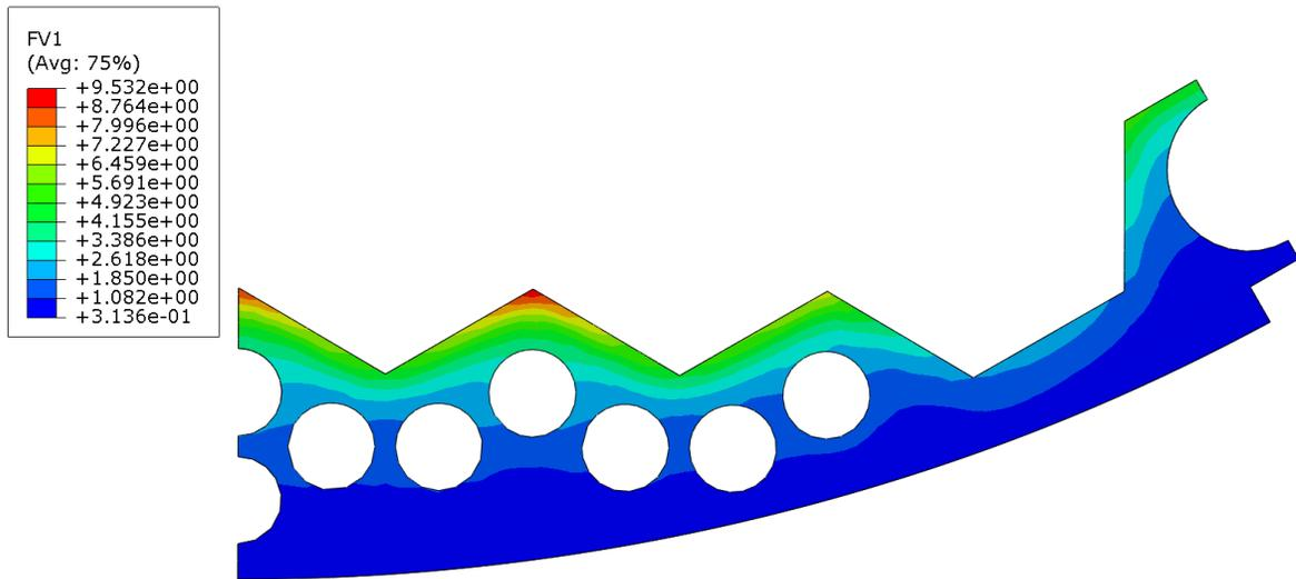
Figure 3. Internal heat sources due to gamma radiation in cross-section with maximum temperature in selected campaign (in  $W/cm^3$ )
