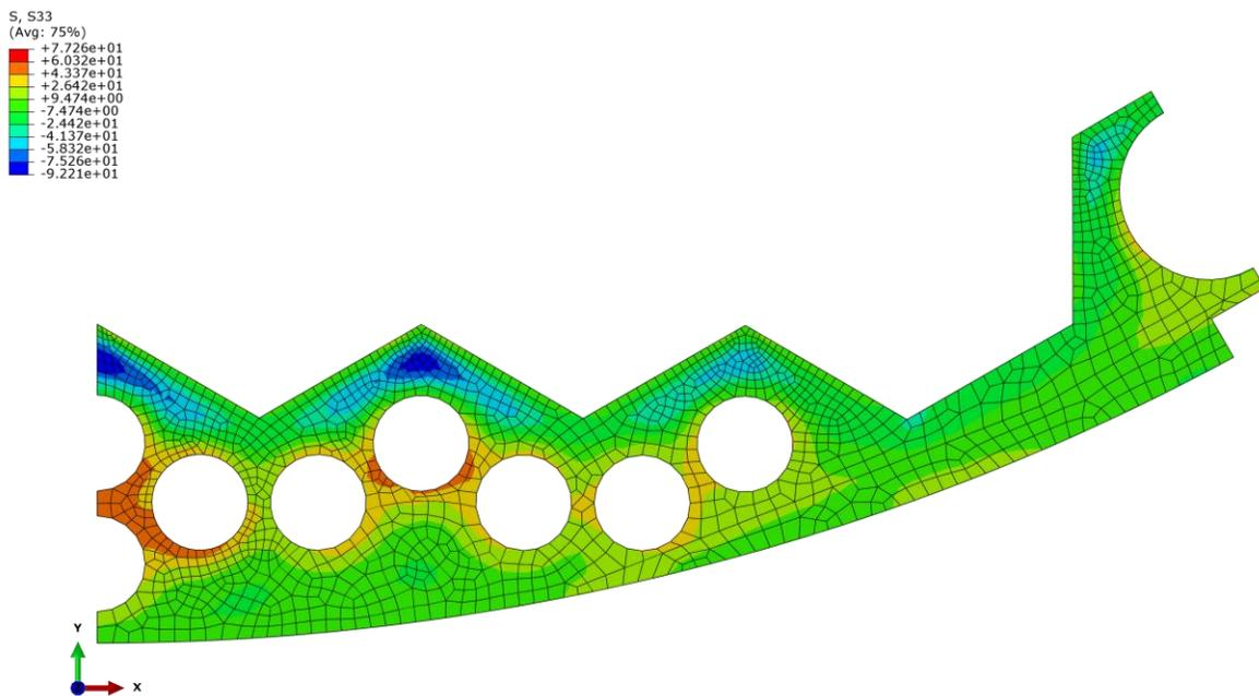
Figure 7. Distribution of axial stress for 60 years of reactor operation, for reactor full power state (in MPa)
