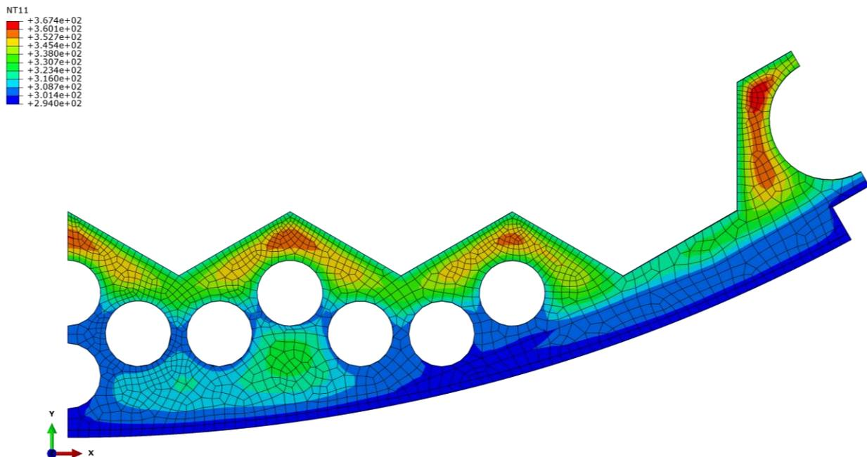
Figure 5. Distribution of temperature in the predicted (selected) campaign for reactor full power state (in °C). Cross-section corresponding to maximum temperature.
