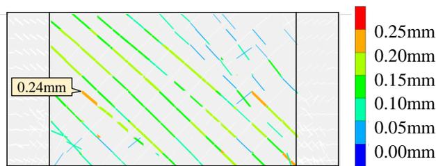
Figure 6. Crack width distribution on FE analysis with DLCM (drift angle  $+0.2\%$ )
