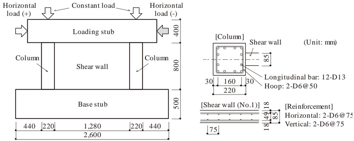
Figure 2. Test specimen of RC shear wall
