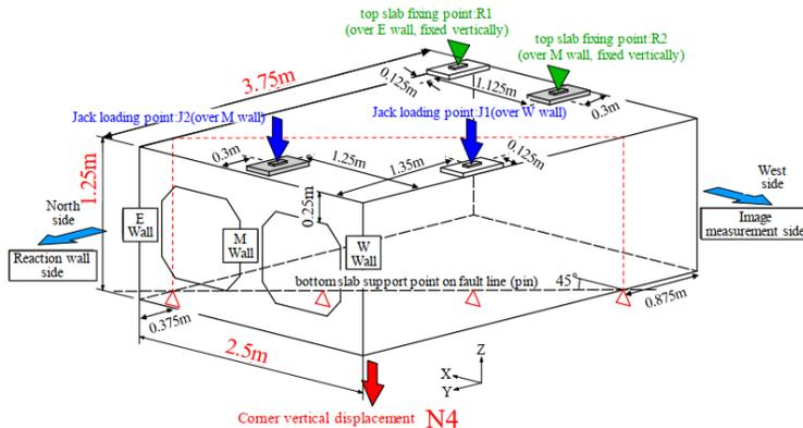
Figure 8. Loading setup
