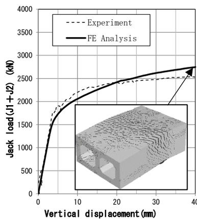
Figure 12. Jack load – Vertical displacement relationships
