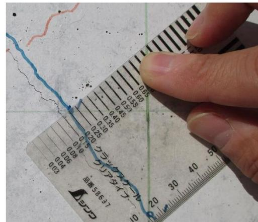
Photo 2. Crack scale
