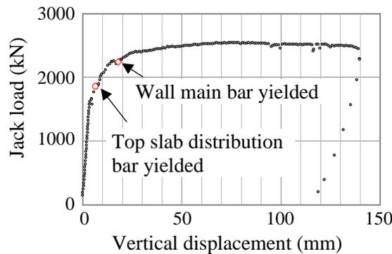
Figure 9. Jack load – Vertical displacement relationship
