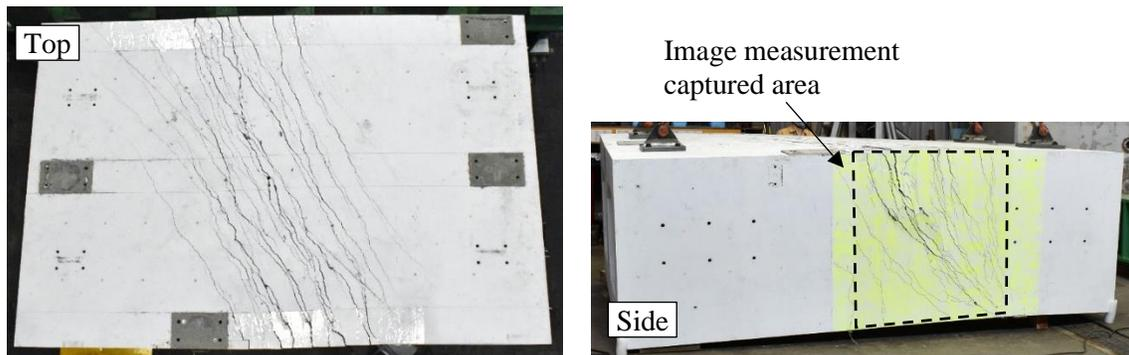
Photo 3. Cracks of test specimen after experiment
