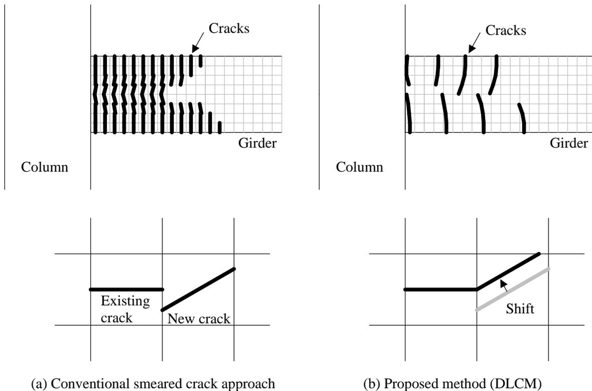
Figure 1. Comparison between conventional smeared crack model and DLCM by Sato et al. (2014)
