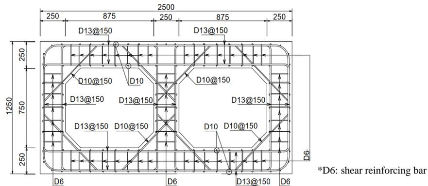
Figure 7. Test specimen of RC box culvert
