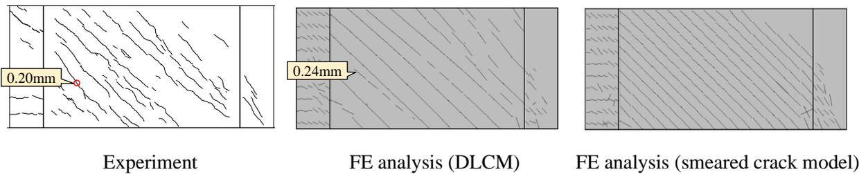
Figure 5. Crack distribution (drift angle  $+0.2\%$ )
