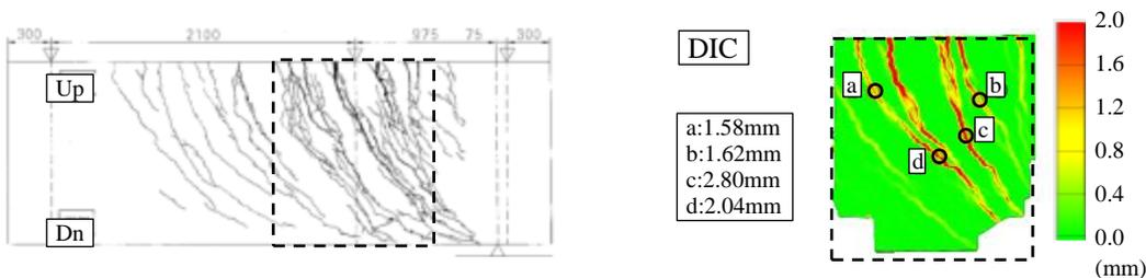
Figure 10. Cracks of test specimen (Experiment vs. image measurement by DIC) (disp. 40mm)
