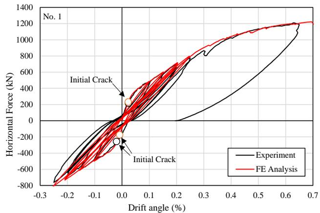
Figure 4. Horizontal force – drift angle relationships
