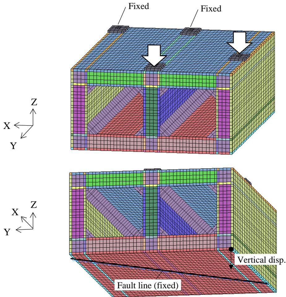
Figure 11. FE analysis model of RC box culvert
