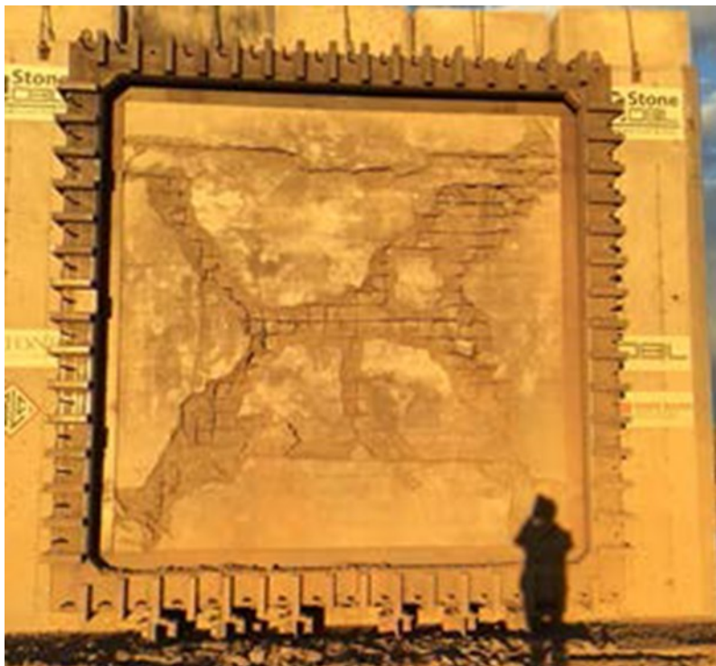
Figure 2. The post-test view of ASME blast test concrete slab
