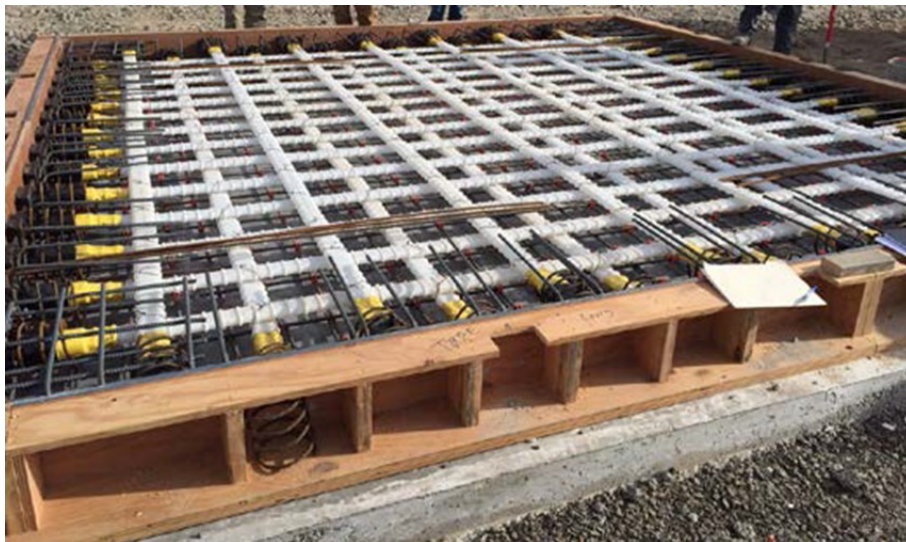
Figure 1. Concrete slab used in ASME blast test
