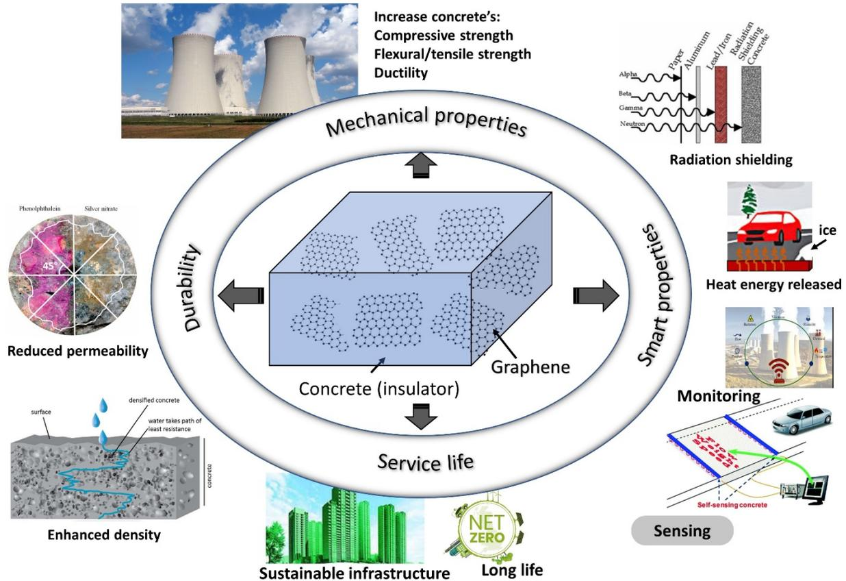
**Figure 1.** Multifunctional concrete with graphene-based materials.
