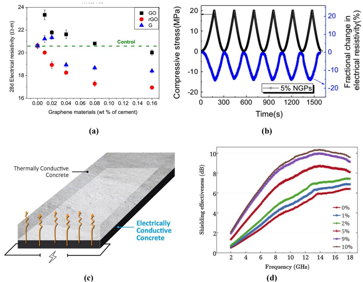
**Figure 5.** Smart functionality: (a) average electrical resistivity of 28-day GCCs, Qureshi and Panesar (2020), (b) Piezoresistive behavior of cement composites infused with 5% graphene under cyclic loading, Sun et al. (2017), (c) Concept of de-icing application on the graphene reinforced concrete pavement, Talga (2018), and (d) Effectiveness of electromagnetic shielding of the cement composites infused with 0%, 1%, 2%, 5%, 9% and 10% graphene, Sun et al. (2017).
