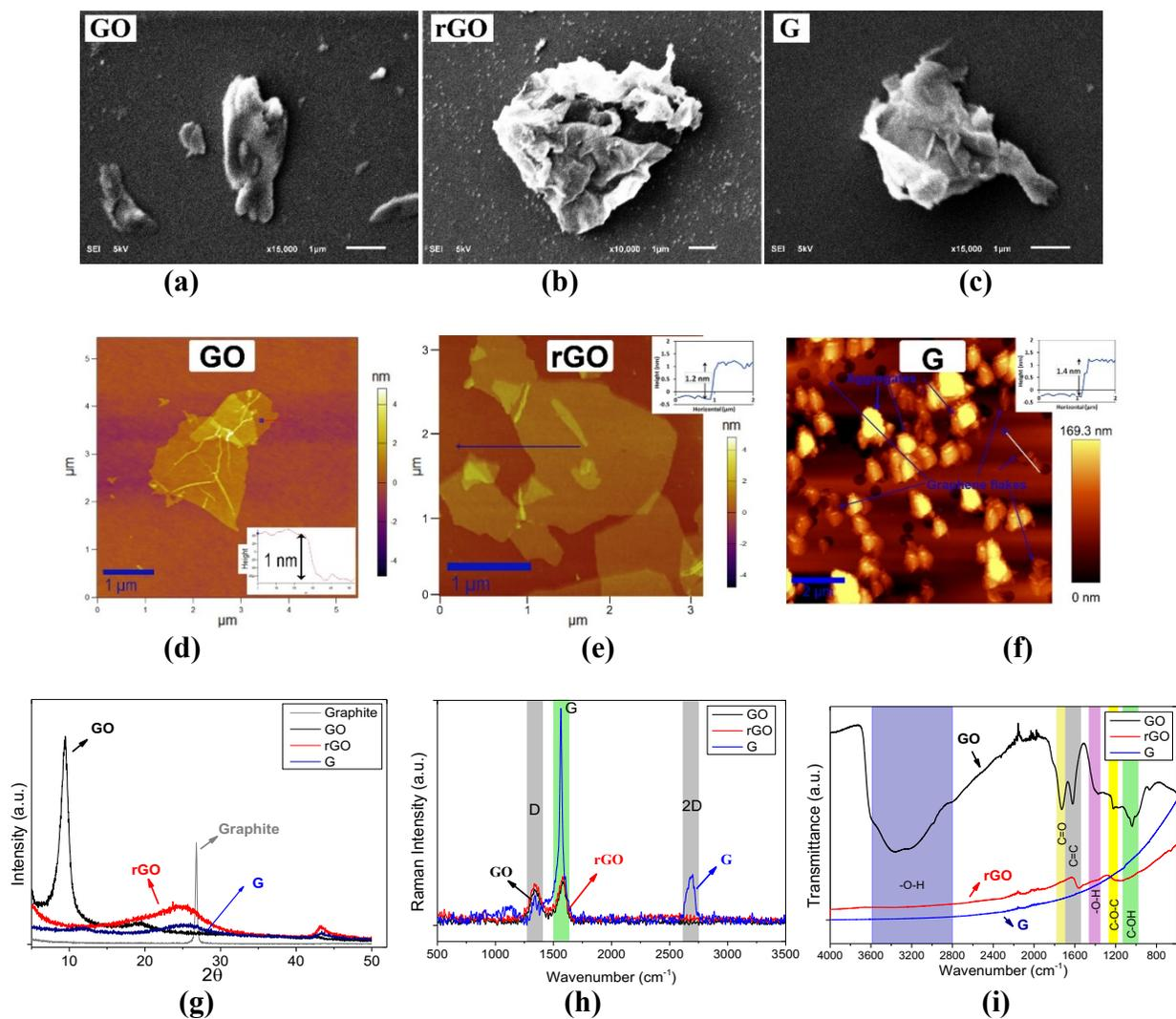
**Figure 2.** Characterisation of graphene materials; SEM images: (a) GO, (b) rGO, and (c) GnP; typical AFM images in water dispersion: (d) GO, (e) rGO, and (f) GnP; (g) XRD pattern, (h) Raman spectroscopy, and (i) FTIR graph, Qureshi and Panesar (2020).
