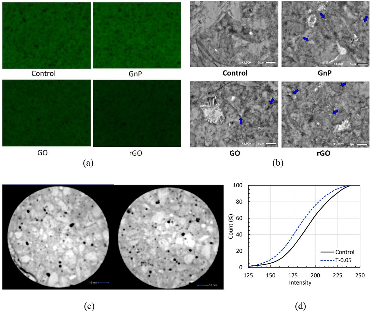
**Figure 6.** Microstructural analysis, graphene-cement paste composite: (a) Fluorescence microscopic image and (b) SEM images, and graphene-cement concrete: (c) CT scan images, and (d) distribution of intensity from CT scan image avoiding coarse aggregate and large pores.
