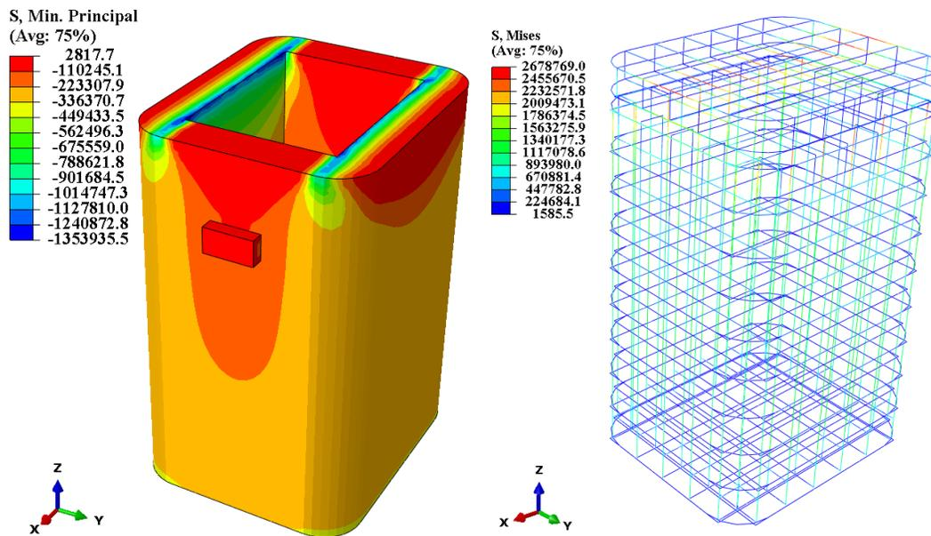
Figure 7. Stress distribution at 50°C (left: UHPC body; right: reinforcement)
