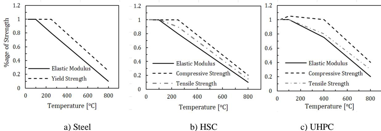
Figure 4. Effect of elevated temperatures on reinforced concrete materials (Model input)
