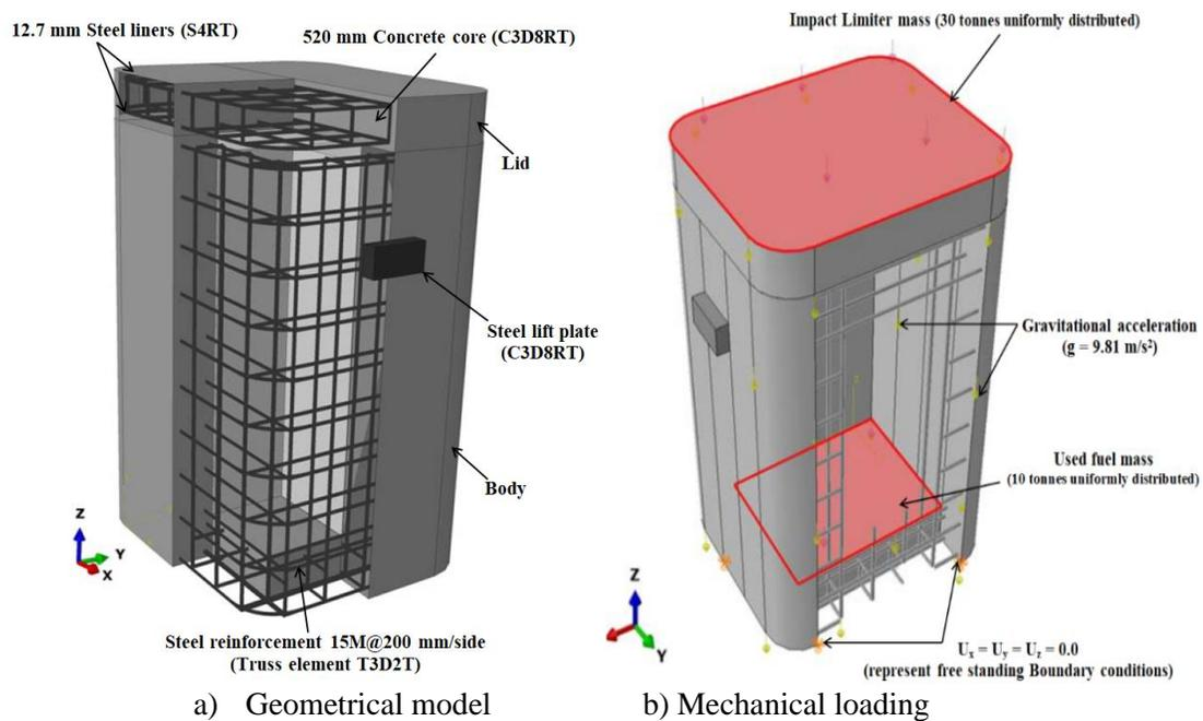
Figure 2. Generated FE model for DSC container (Case study).
