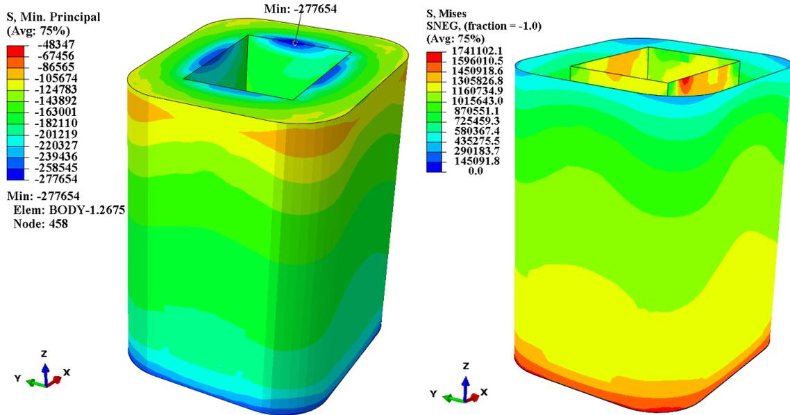
Figure 5. Maximum compressive stress at 50°C (left: HSC core; right: steel liners).
