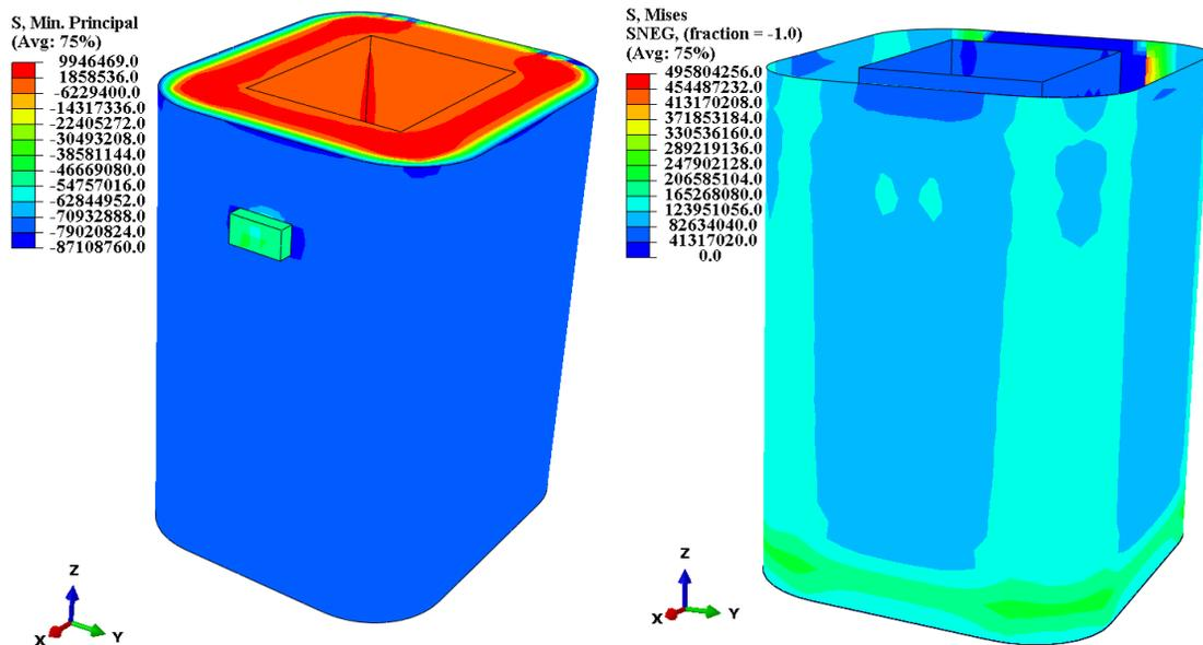
Figure 6. Stress distribution at 800°C (left: HSC core; right: steel liners)
