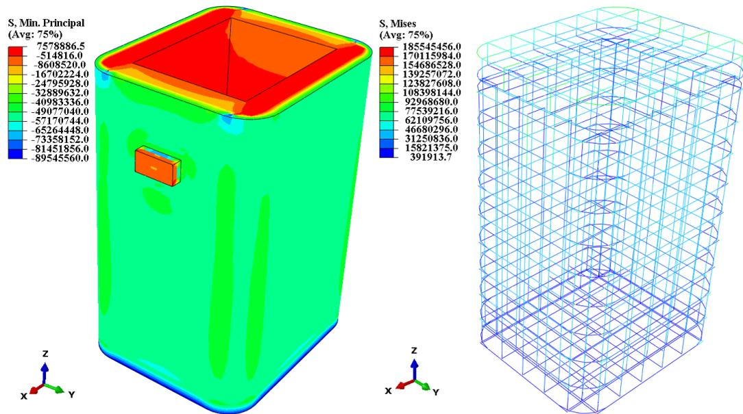
Figure 8. Stress distribution at 800°C (left: UHPC body; right: reinforcement)
