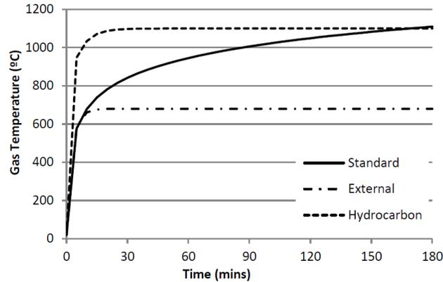
Figure 3. Temperature - time histories of the standard, external and hydrocarbon fires.
