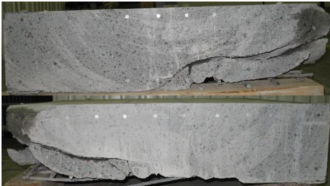
Figure 6. Vertical and horizontal mid-sections of the slab after IRIS 2010 P1 test.
