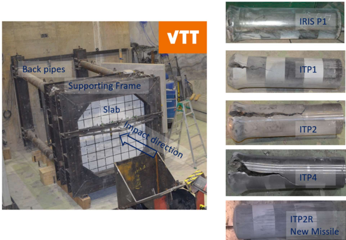
Figure 1. Test setup (left) and deformed projectiles after tests (right)
