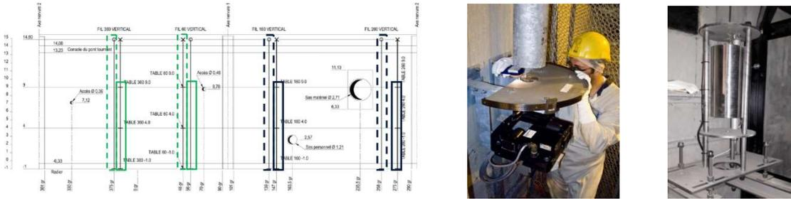
Figure 6. Location of the considered pendulums/invar wires (left) and figures of the used devices (right)
