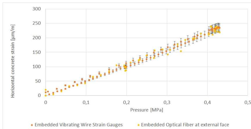
Figure 5. Concrete strain measured with VWSG and Embedded Optical Fiber [ $\mu\text{m}/\text{m}$ ] versus pressure - mid height of the containment - VD5 pressure test
