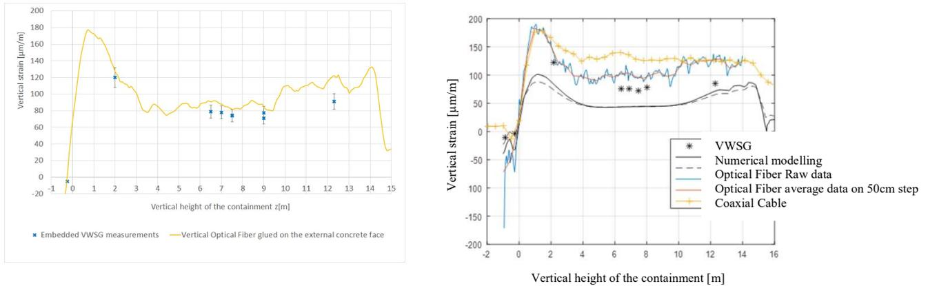
Figure 8. Vertical concrete strain measured with VWSG and glued optical fiber during VD5 pressure test (left) - Vertical concrete strain measured with VWSG, glued optical fiber and coaxial cable during VD3 pressure test (right)
