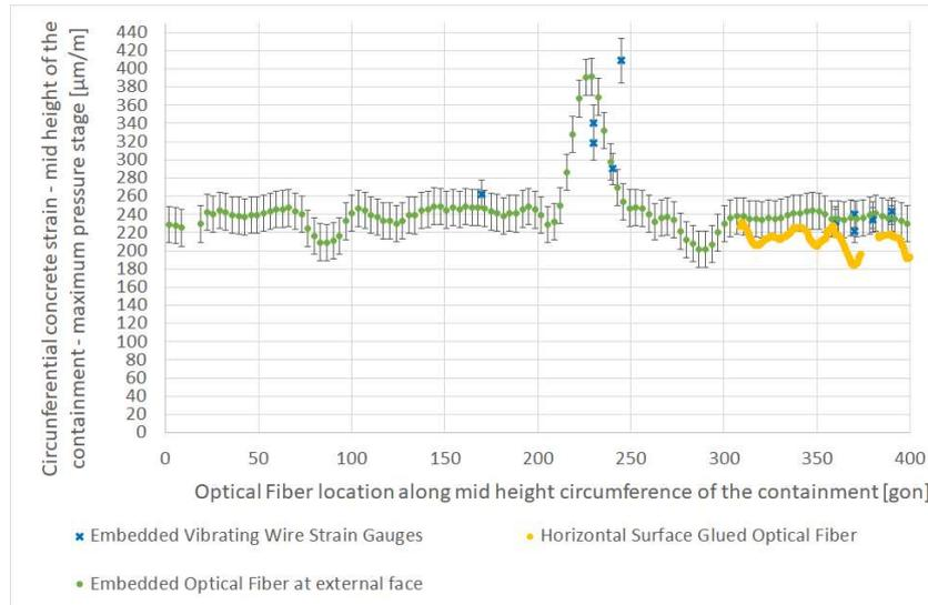
Figure 4. Circumferential concrete strain measured with VWSG, Glued and Embedded Optical Fiber [ $\mu\text{m}/\text{m}$ ]- mid height of the containment - maximum pressure stage during VD5 pressure test
