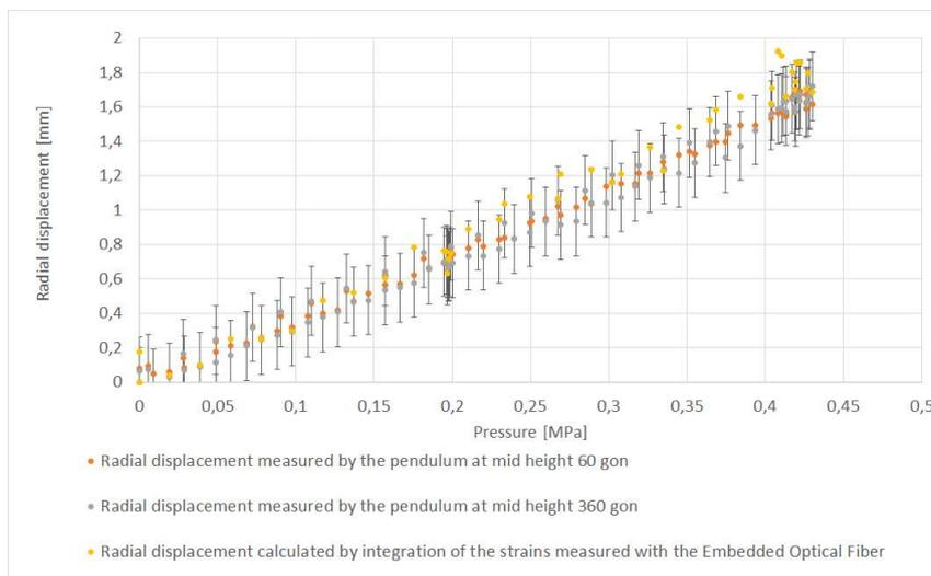
Figure 7. Concrete strain measured with Embedded Optical Fiber integrated over the length [mm] versus pressure – comparison to mid height pendulums - VD5 pressure test
