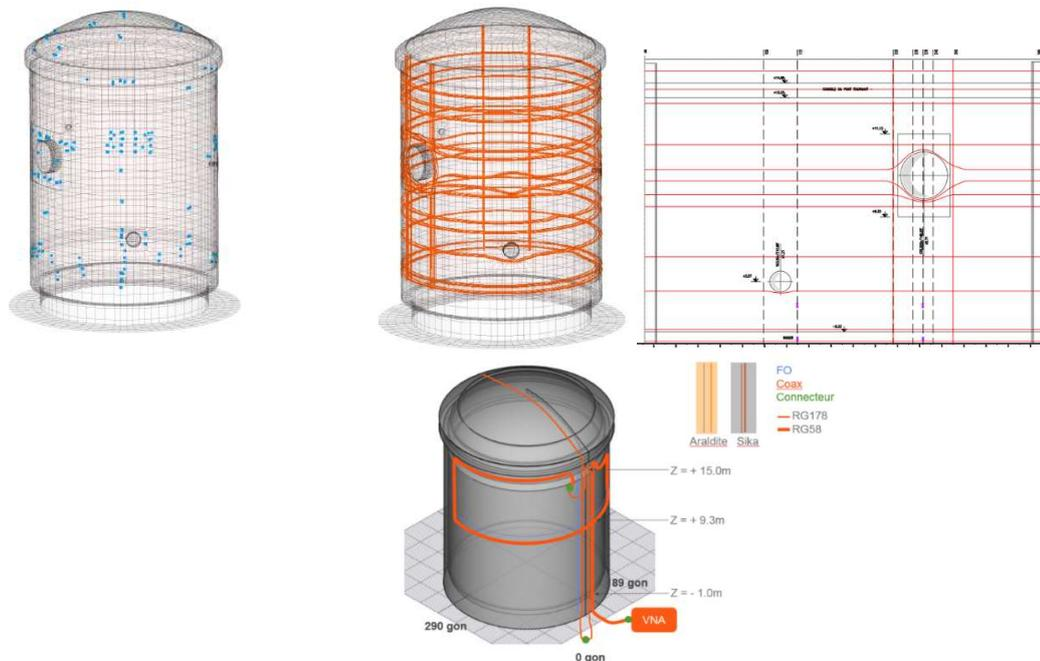
Figure 1. Local and distributed concrete strain measurement on Vercors Mockup – embedded devices at the top (VWSG at the left and Optical Fiber on the right) and glued on the external face devices at the bottom (Optical Fiber and Coaxial Cable)
