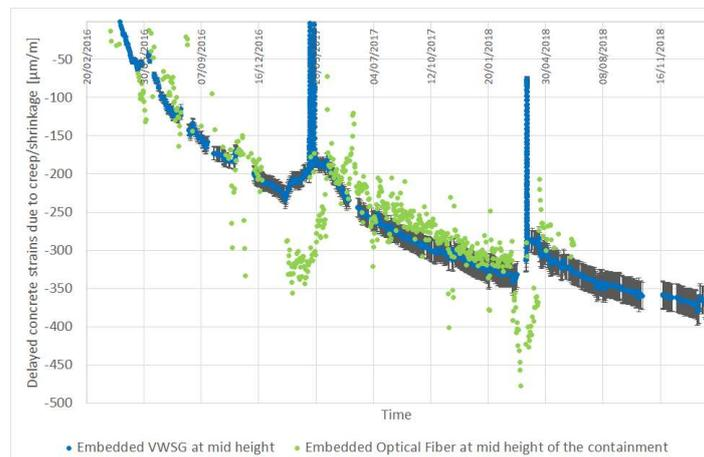
Figure 9. Delayed concrete strains due to creep/shrinkage measured by the embedded optical fiber compared to Vibrating Wire Strain Gauges
