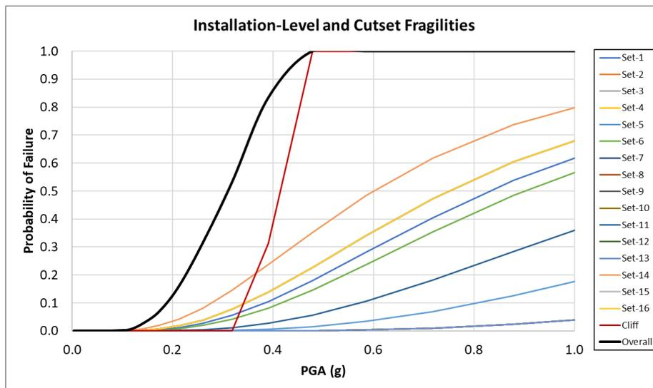
Figure 1. Example installation-level fragility with potential cliff edge failure (IAEA, 2022).
