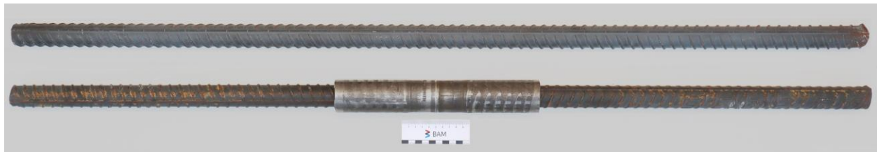
Figure 4. Exemplary reference bar of 32 mm and 32 mm reinforcement bar with coupler before high-speed tensile tests (e.g. Dextra GRIPTEC Standard Splice G32).
