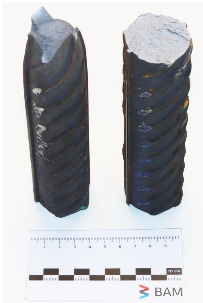
Figure 8. Fracture surfaces of a 40 mm rebar after high-speed tensile test with ductile failure (left) and brittle failure (right).
