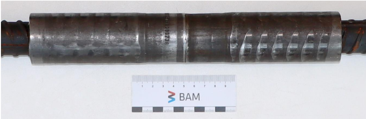
Figure 1. Exemplary reinforcement bar of 32 mm with mechanical splicing system (e.g. Dextra GRIPTEC Standard Splice G32).
