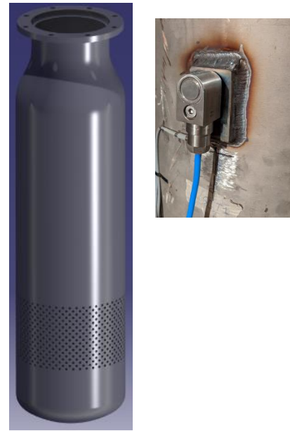
Figure 2: sparger and accelerometer on the sparger support
