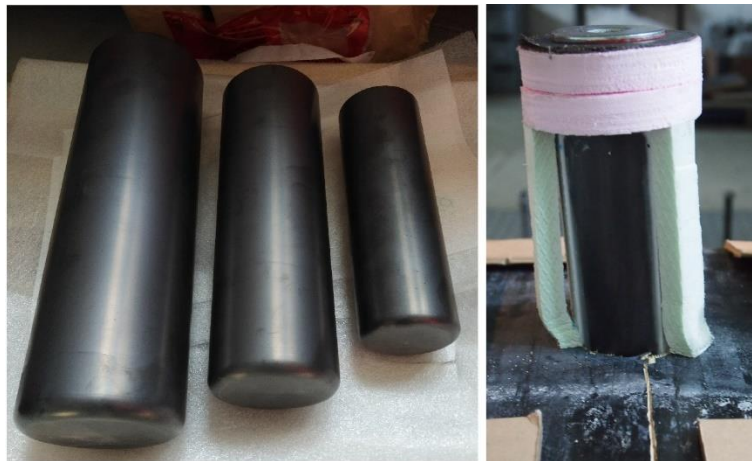
Figure 1. Scaled impactors (left) and impactor with sabot during a preliminary test (right), photos: F. Bracklow
