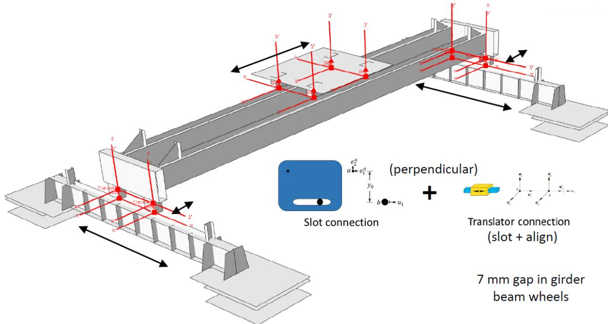
Figure 6. Connectors representing the wheel interactions, including gaps
