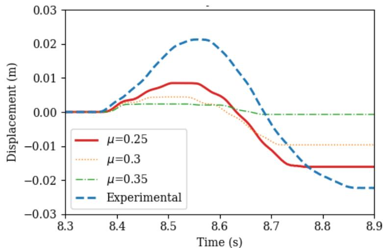
Figure 4. Transient analysis for calibration of friction wheel/runway (run 62)
