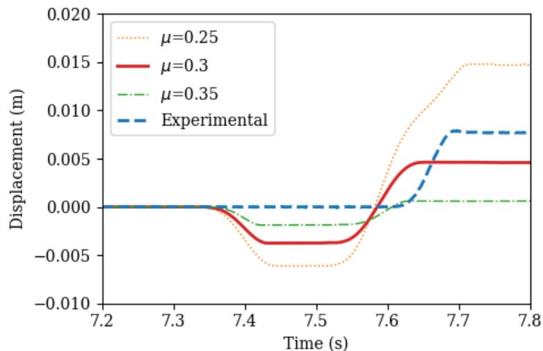
Figure 5. Transient analysis for calibration of friction wheel/girder (run 64)
