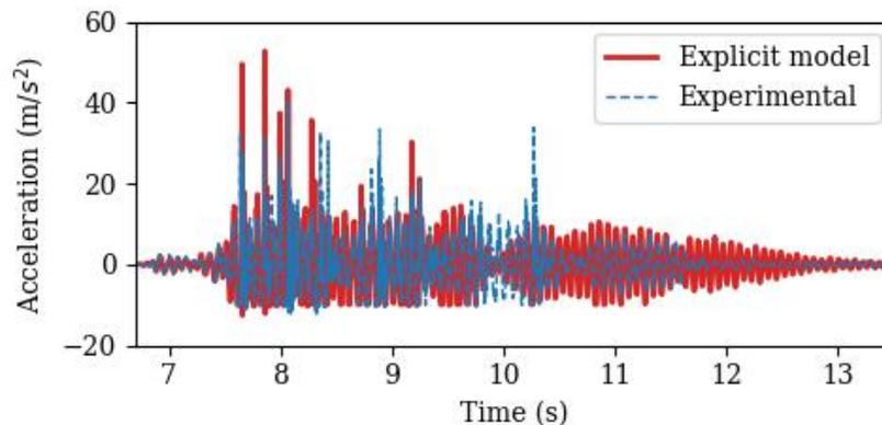
Figure 8. Vertical acceleration of the chariot for run 53
