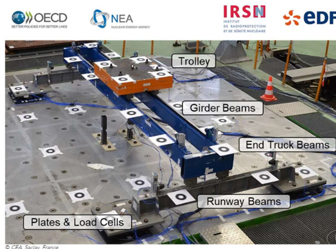
Figure 1. Overhead crane mock-up on the shaking table
