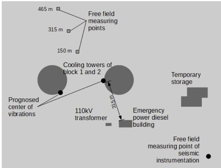
Figure 6. Schematic site plan of critical buildings/components of NPP
