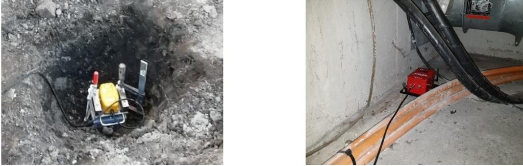
Figure 1. typical sensor installations (left: free-field measuring point, coupling to soil by ground spike according to DIN 45669-2; right: measuring point on foundation, loose installation)
