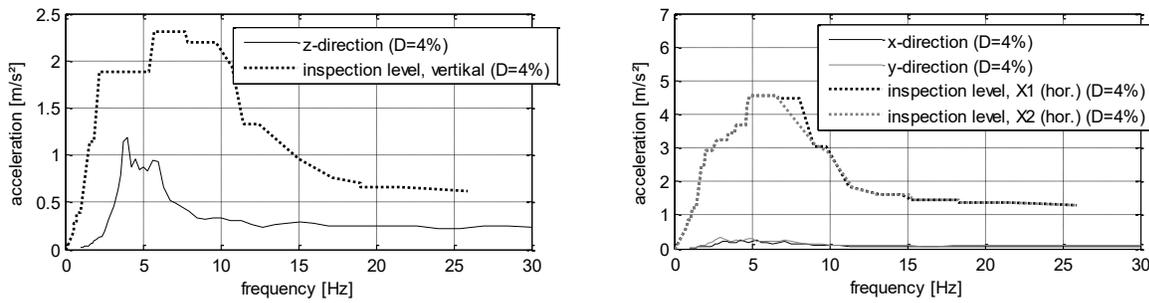
Figure 8. Comparison of vibration response spectra with inspection level at foundation of emergency power diesel building, D = 4 % (left: vertical direction, right: horizontal direction)
