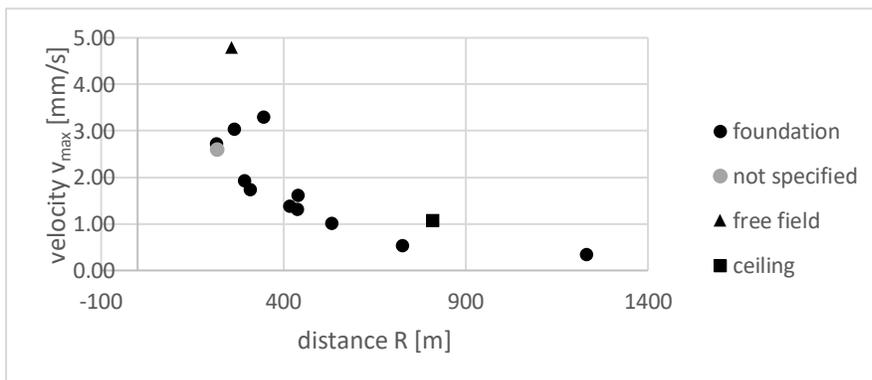
Figure 5. Maximum velocities during blast demolition of a cooling tower of power plant Lünen
