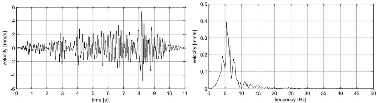
Figure 3. Velocity measured at 100 m distance in vertical direction (left: time history, right: spectrum of measured velocity by FFT)
