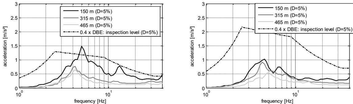
Figure 7. Comparison of free-field response spectra with inspection level, D = 5 % (left: vertical direction, right: horizontal direction – spreading direction)
