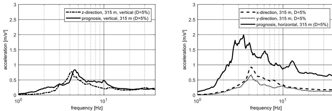
Figure 9. Comparison of vibration response spectra with vibration prognosis and inspection level of NPP, D = 5 % (left: vertical direction, right: horizontal direction)
