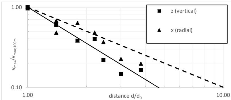
Figure 4. Reduction of maximum velocities with increasing distance (related to MP at  $d = 100$  m)
