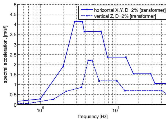
Figure 3. Response spectra ( $D = 2\%$ ) of 110 kV-plant feeding transformer at installation location
