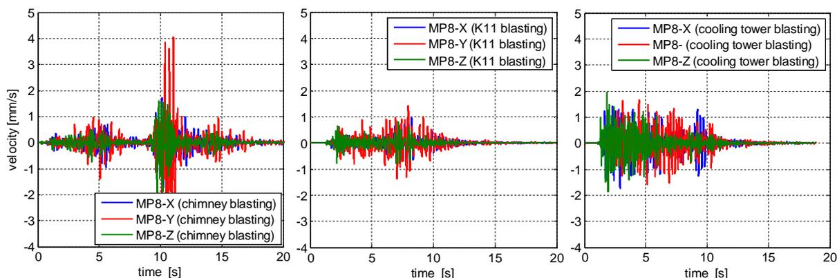
Figure 8. Velocity recordings at the foundation of switchgear building during all three blastings
