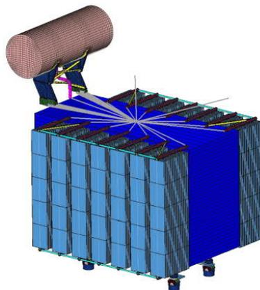
Figure 4. FE-model of the transformer
