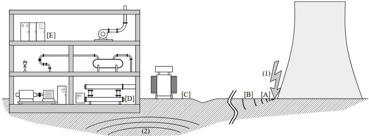
Figure 1. Equipment under short-term ground vibration loading: e.g. near-site demolition (1), impacts during decommissioning (1); earthquake loading (2)
