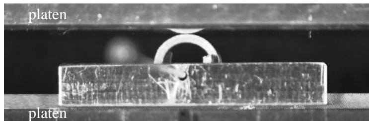
Figure 8. Single coil specimen installed in the test rig
