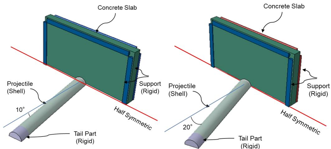
Figure 2. Overview of Numerical Simulation Model for IB1,3 (left) and IB2,4 (right).
