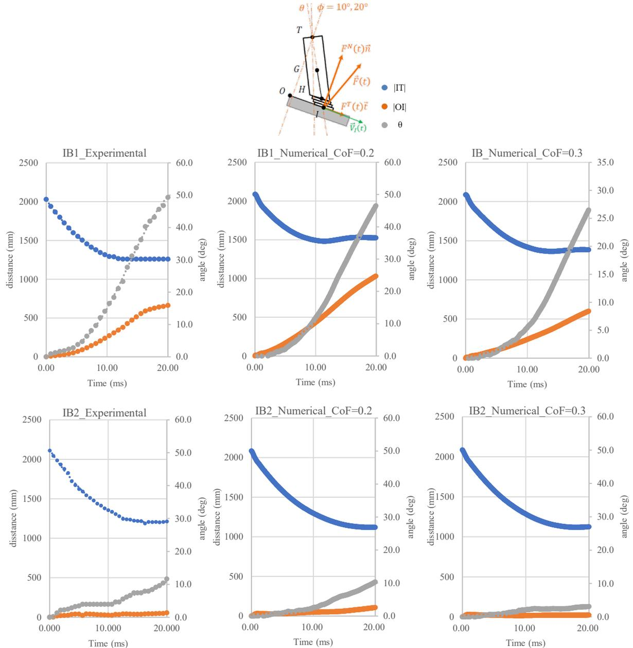
Figure 7. Comparison of Kinematic Data of the Projectiles; Experimental (Left), Numerical Cof = 0.2 (Center), and Numerical Cof = 0.3 (Right)
