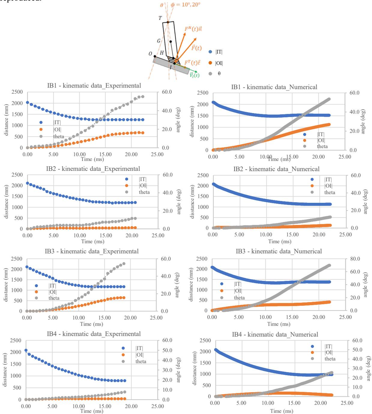
Figure 5. Comparison of Kinematic Data of the Projectiles; Experimental (Left) and Numerical (Right).
