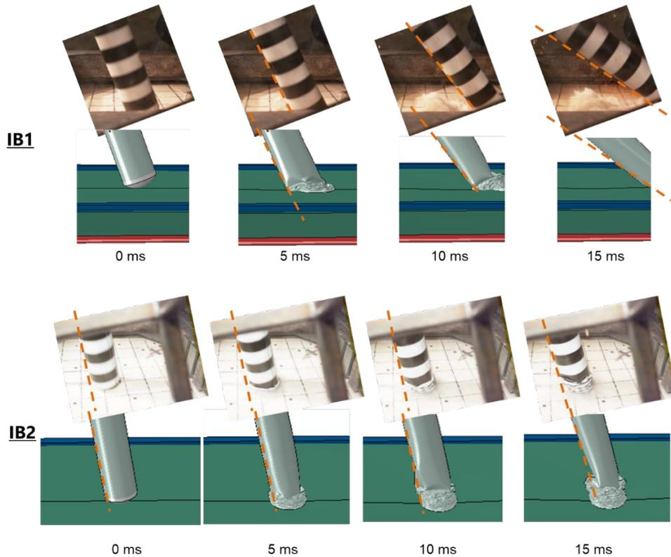
Figure 3. Behavior of the projectile in IB1(Upper) and IB2(Lower).
