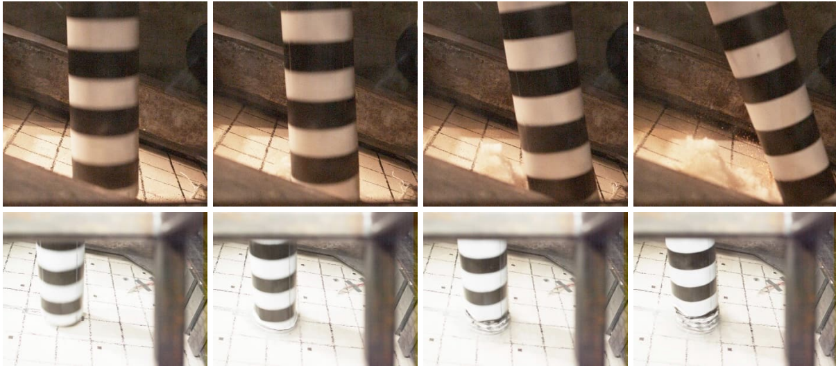
Figure 3. Top view of the impact in tests IB1 (top) and IB2 (bottom). Time moments: frame 1: 0 ms; frame 2: 3.7 – 3.75 ms, frame 3: 7.4 – 7.5 ms and frame 4: 11.1 – 11.3 ms.
