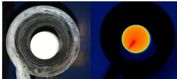
Figure 10. Photo of a disc-shaped steel specimen with a ceramic coating on top placed in an inductive heating device (on the left) and thermal image of the specimen after heating by an additional laser pulse (on the right). A partial delamination (linear flaw) of the coating is clearly visible on the thermal image, although it is not visible on the photo.
