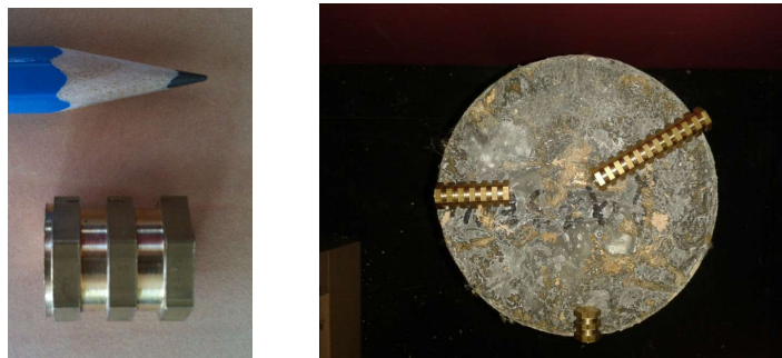
Figure 10: Tests performed with different anchorage length of the LVDT system (16mm which is the reference of the previous 6 samples, 40mm and 70mm)
