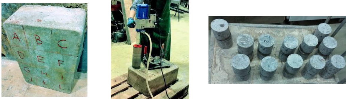
Figure 2. Drilling of core from the concrete slab cast of the concrete used in the wall concrete and stored in the same condition.
