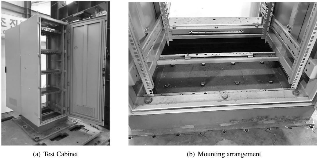
Figure 2. Test setup for shake table experiment
