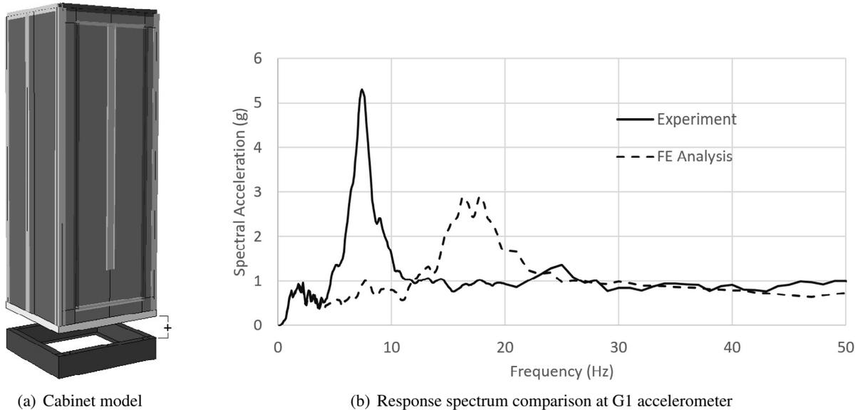
Figure 6. Modeling cabinet with additional channel section
