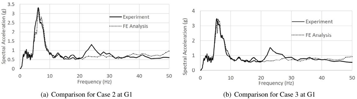
Figure 12. Response spectrum comparison for Case 2 & 3 using approach 3
