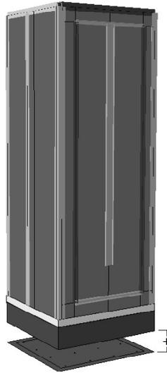
Figure 7. Modeling cabinet with added channel and base plate
