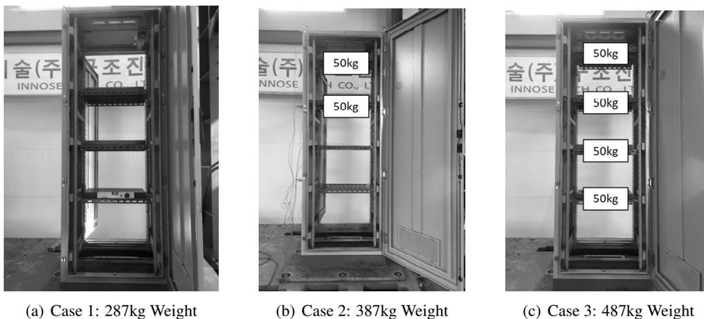
Figure 3. Test setup for different cases
