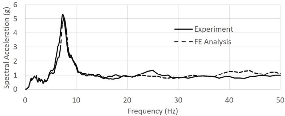
Figure 9. Response spectrum comparison at G1 accelerometer using reconciled modeling approach
