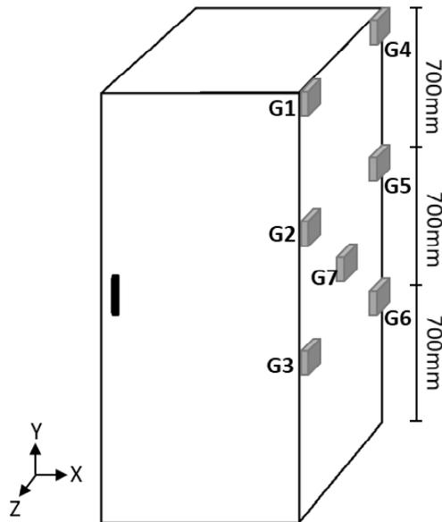
Figure 1. Accelerometers mounted on test cabinet
