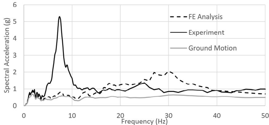
Figure 5. Response spectrum comparison at G1 accelerometer using first modeling approach
