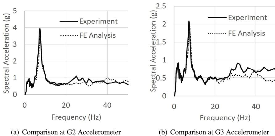
Figure 10. Response spectrum comparison at G2 and G3 accelerometers using approach 3
