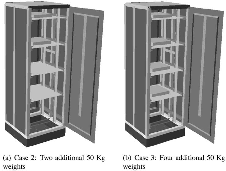
Figure 11. Cabinet FE model for different cases
