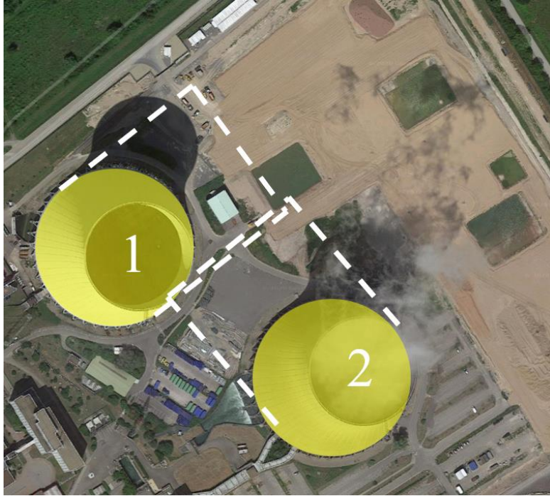
Figure 1 The two cooling towers (yellow) of Philippsburg powerplant and predicted debris area after dismantling
