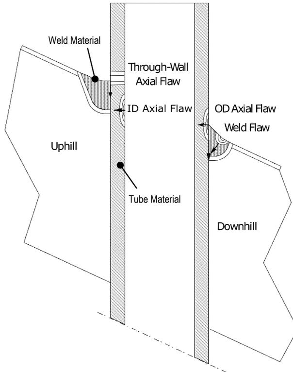
Figure 2. SCC initiation sites and crack shapes modelled in JASPER
