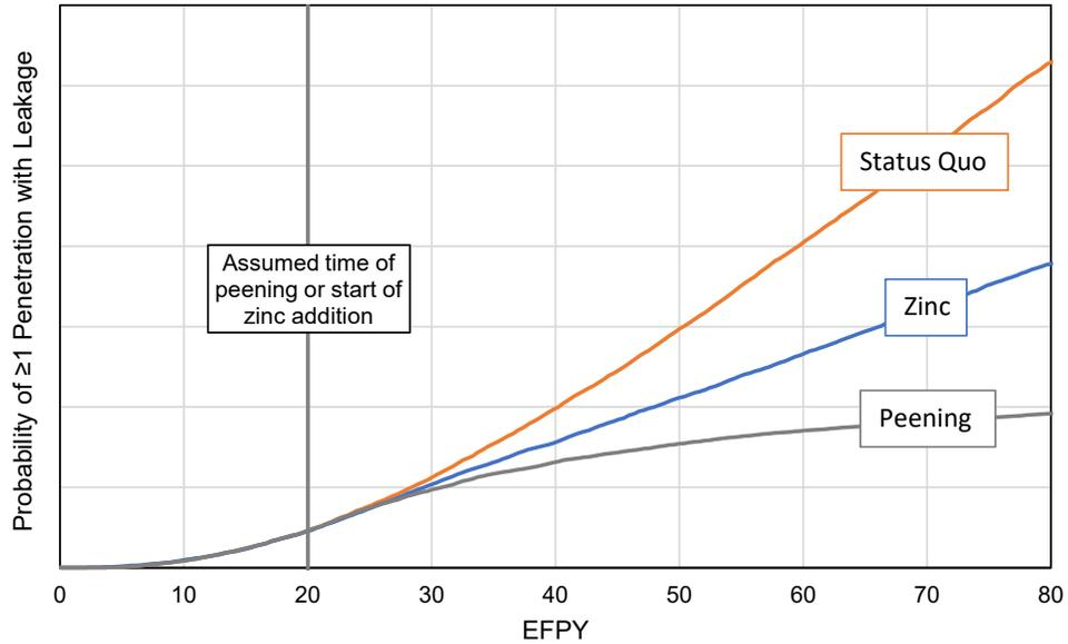
Figure 4. Example results – probability of leakage
