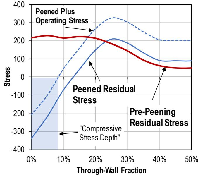
Figure 1. Illustrative comparison of stress profiles with the application of peening
