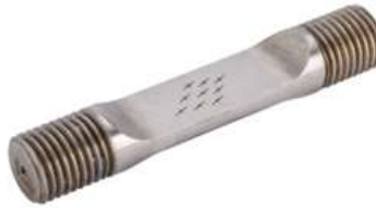
Figure 5. Typical specimen for the investigation of artificial crack fields from 22NiMoCr3-7.
