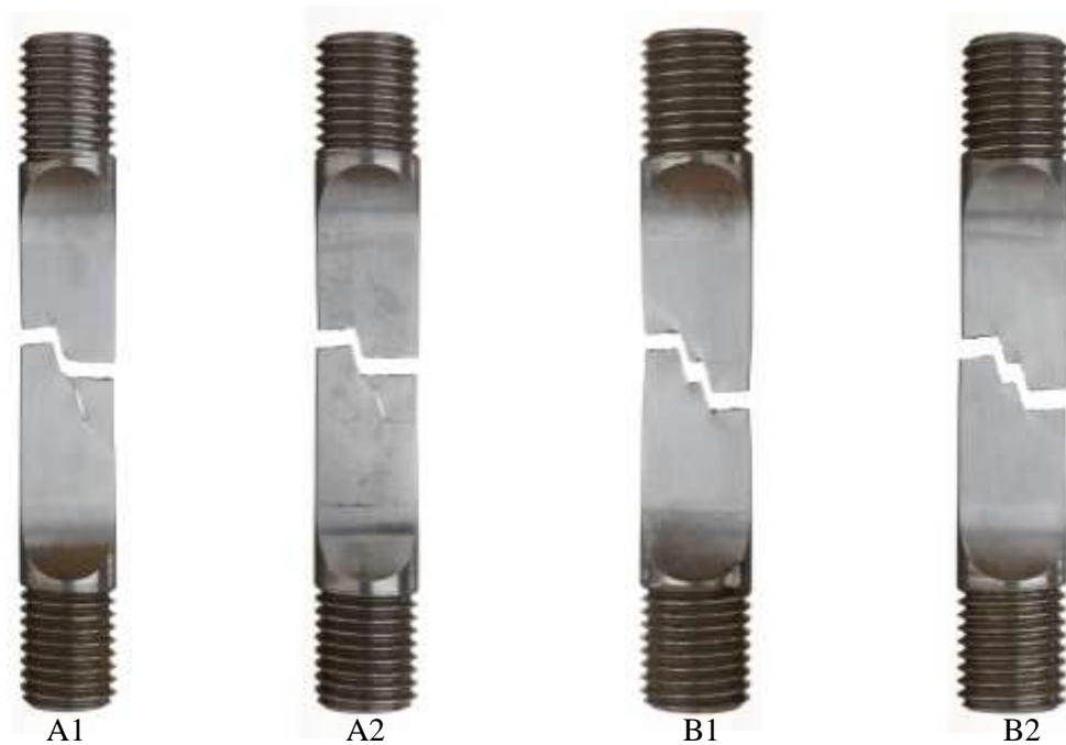
Figure 8. Fractured flaw field specimen; A1: Flaw configuration A at T = -60^\circ\text{C} ; A2: Flaw configuration A at T = -100^\circ\text{C} ; B1: Flaw configuration B at T = -60^\circ\text{C} ; B2: Flaw configuration B at T = -100^\circ\text{C} .
