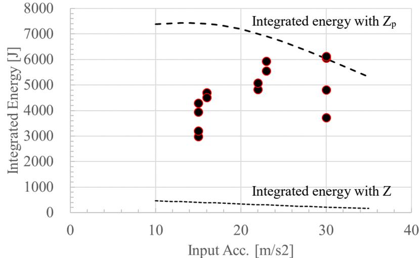
Figure 9. Relationship between integrated energy at failure and input acceleration.
