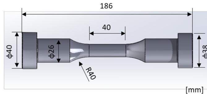
Figure 5. Dimensions of a test specimen.
