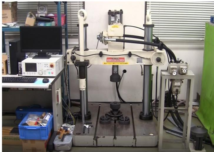
Figure 7. Appearance of a fatigue test machine.
