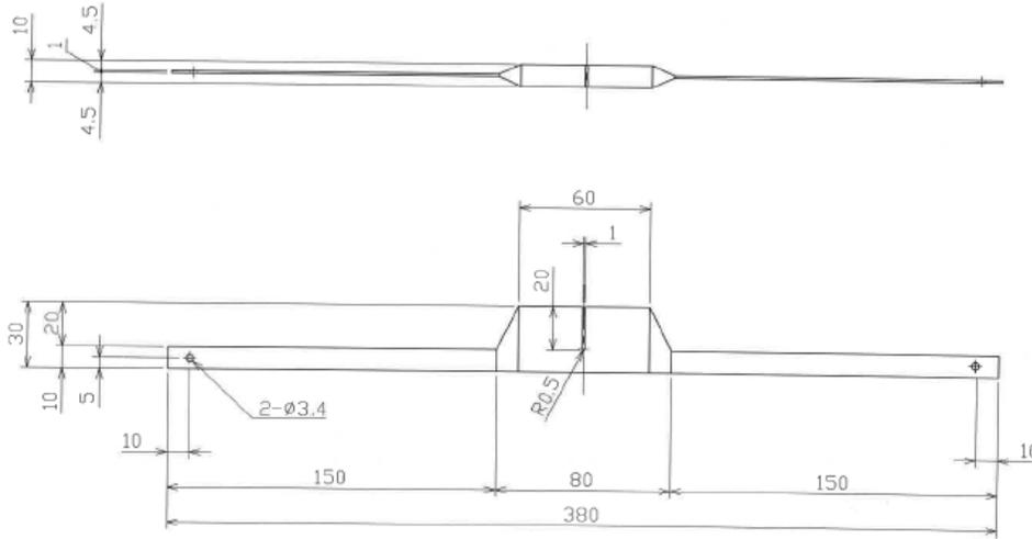
Figure 1. Dimension of specimen for vibration test.
