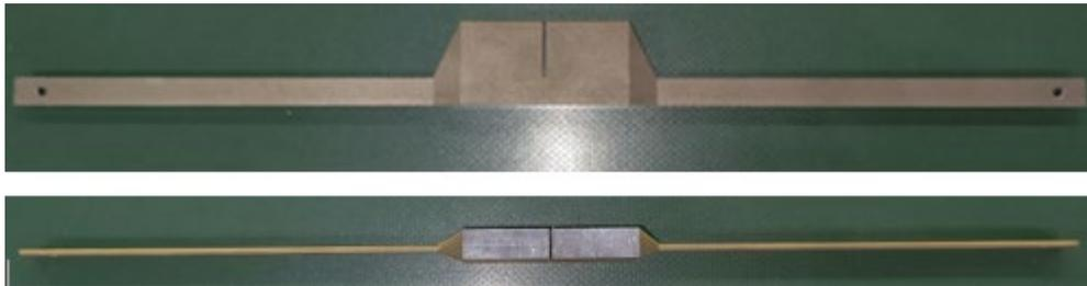
Figure 2. Picture of test specimen for vibration test.
