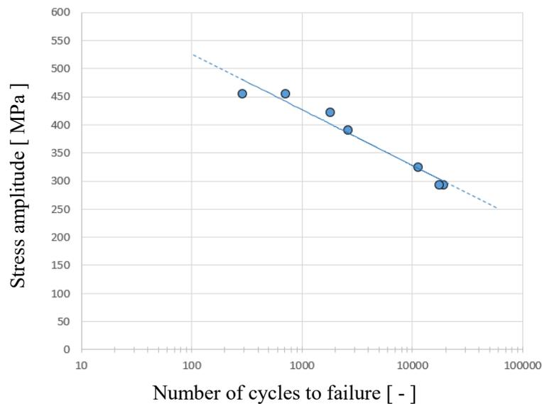
Figure 8. S-N curve of fatigue tests.
