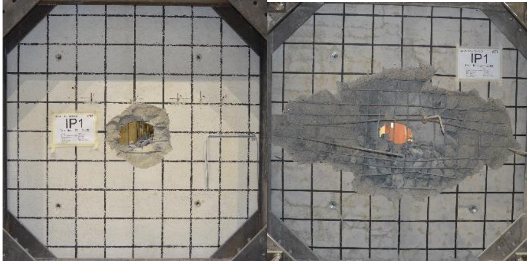
Figure 4. Front and back surfaces of the slab after test IP1 (20 degrees).
