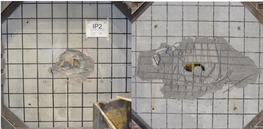
Figure 5. Front and back surfaces of the slab after test IP2 (30 degrees).
