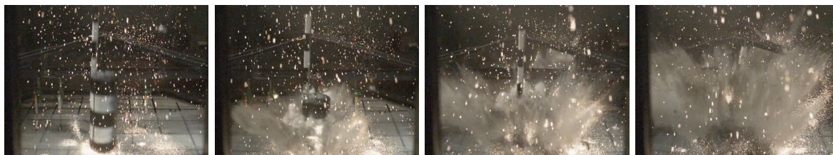
Figure 3. Top view photos of the impact ITP4RR at the moment of the impact and 2.5, 5.0 and 7.5 ms after that.
