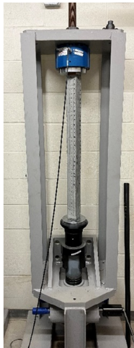
Figure 1: Test specimen loaded into creep frame
