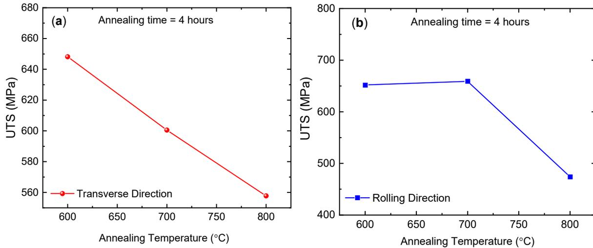
Figure 2. Effect of ultimate tensile strength (UTS) on annealing temperature (a) along the transverse direction, and (b) along the rolling direction. The annealing time is 4 hours.
