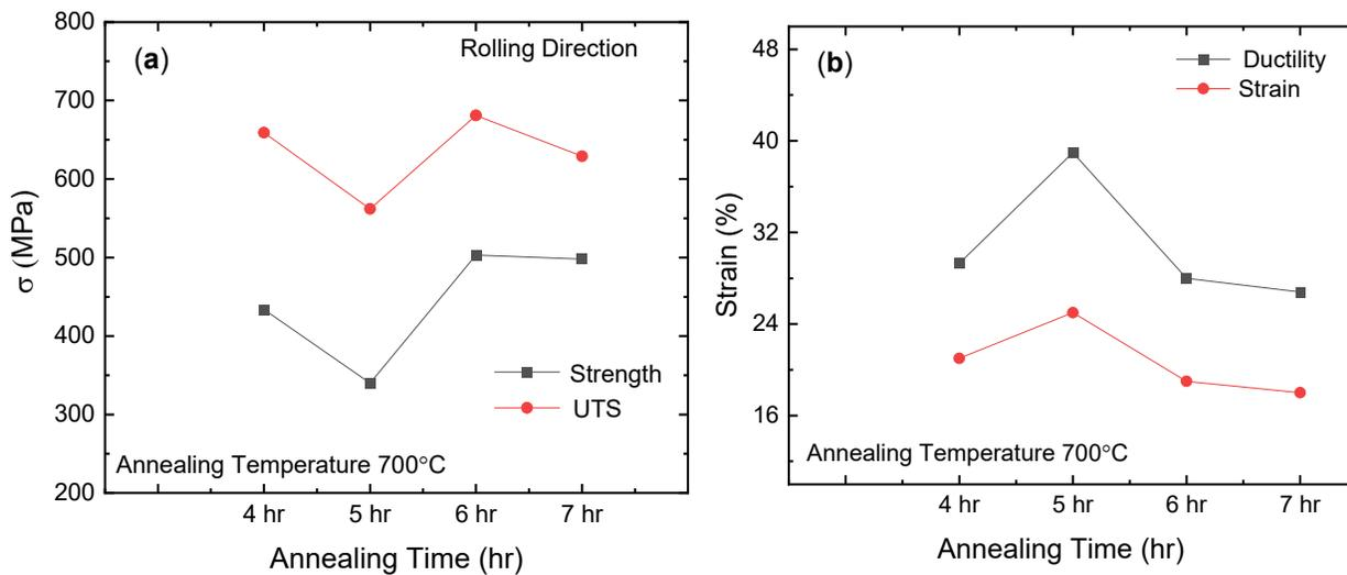
Figure 1. Effect of annealing time on (a) the mechanical strength, and (b) ductility of FeCrAl APMT alloy at 700°C. The yield strength and UTS of the as-received samples without annealing are 570 MPa and 719 MPa, respectively, corresponding to 29% ductility and 19% strain, respectively.
