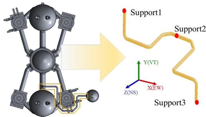
Figure 1. Schematic diagram of target piping system.
