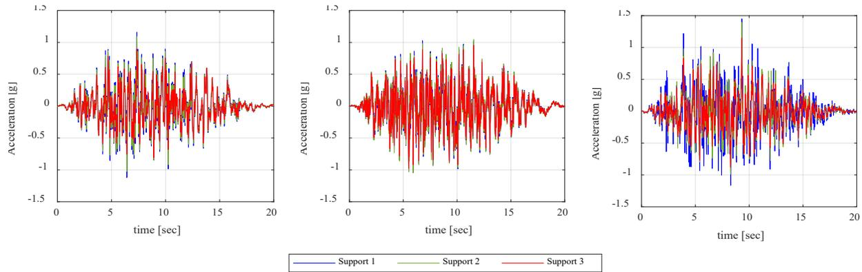
Figure 2. 3-axis input acceleration data on each support.
