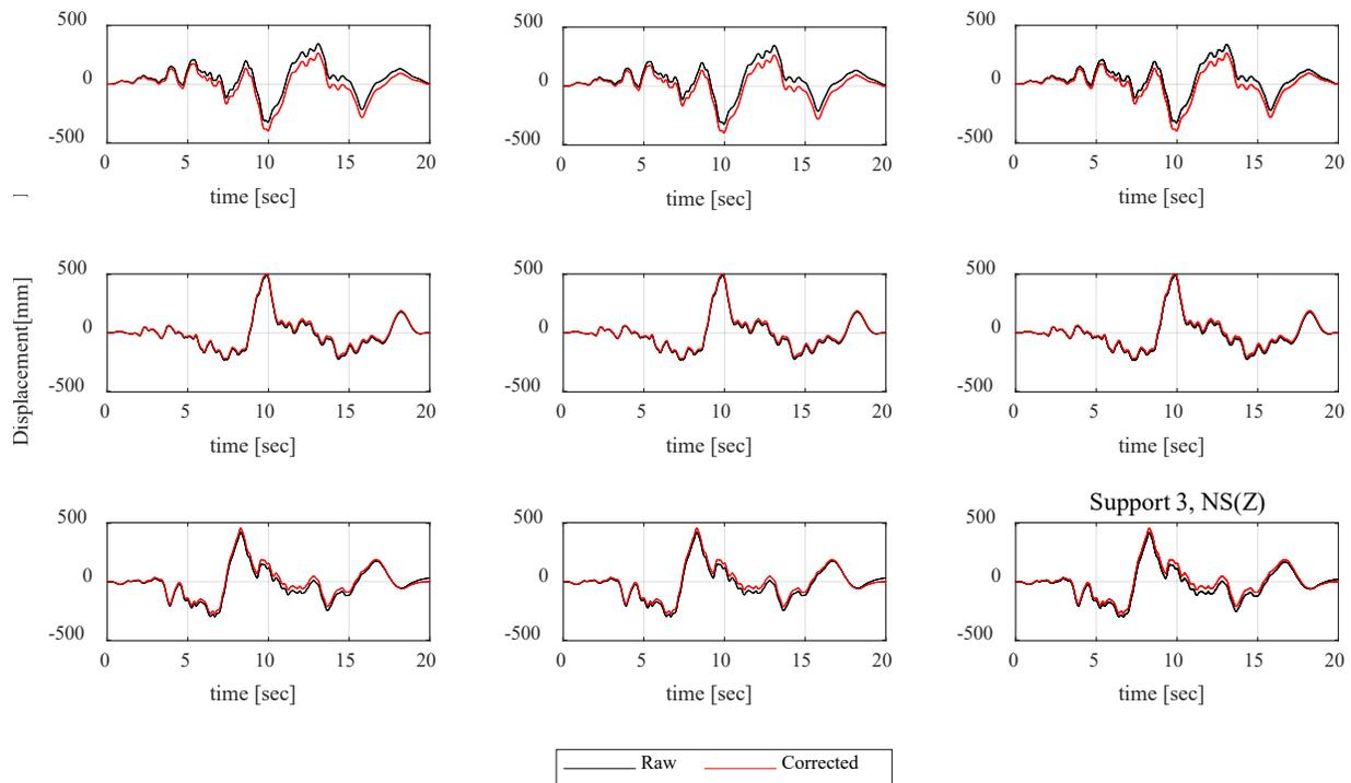
Figure 3. Generated time-historical displacement data using baseline correction
