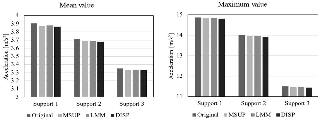
Figure 3. Comparison of the generated acceleration on each support according to the methods.
