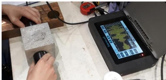
Figure 3. Ultrasonic measurement equipment
