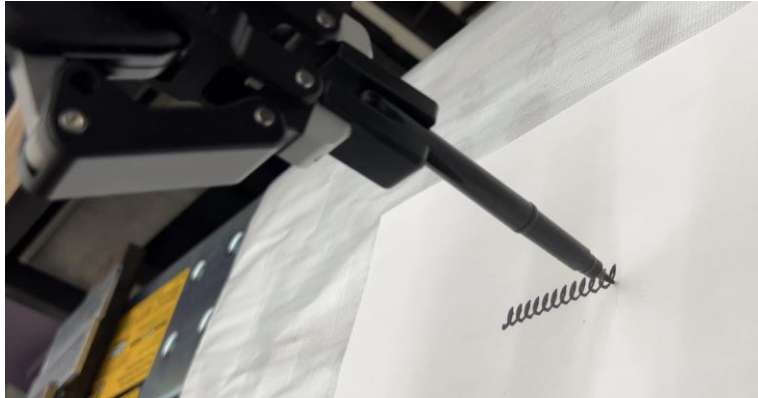
Figure 7. Robotic arm operation for creating weaving pattern with brush pen
