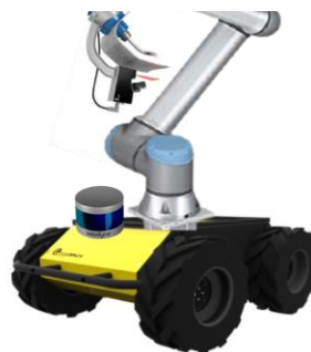
Figure 8. Conceptual design of complete mobile welding robot
