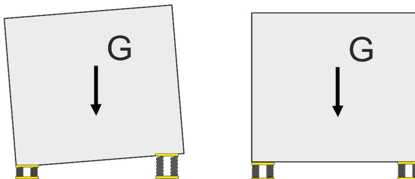
Figure 2. Tilting (exaggerated) of structure (left) due to non-uniform vertical displacement, optimized layout (right).
